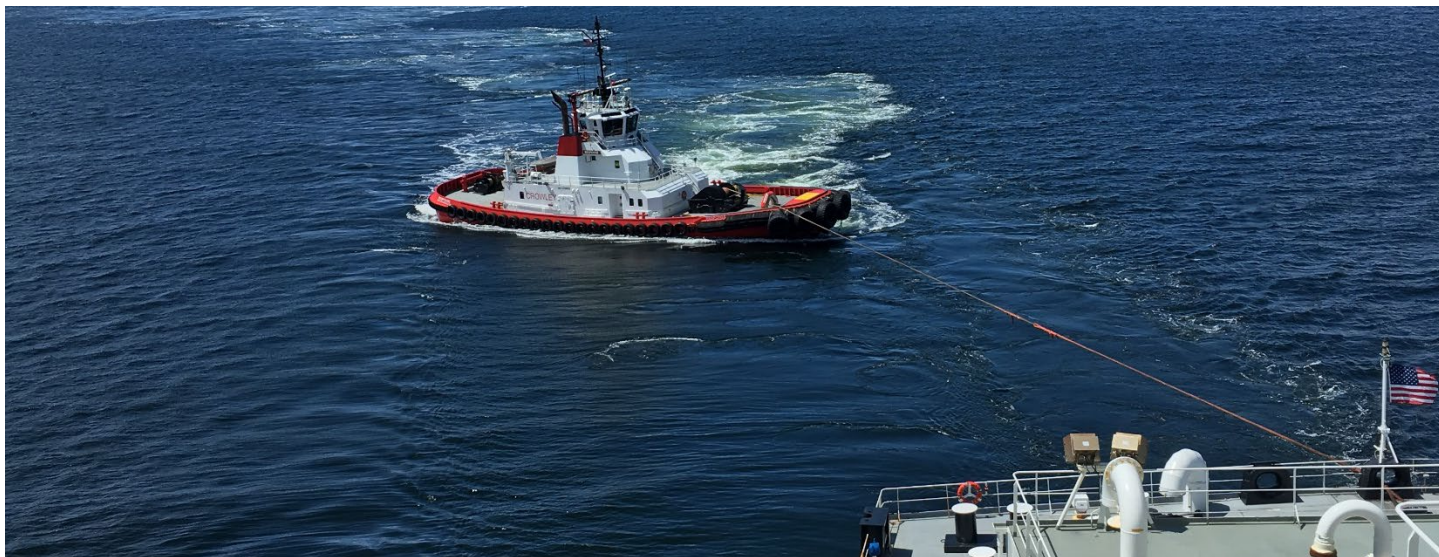
A tug boat and an oil tanker practice emergency assistance maneuvers. The goal of this maneuver is for the tug to stop the forward movement of the oil tanker. This maneuver would be used if the oil tanker had a loss of propulsion.
