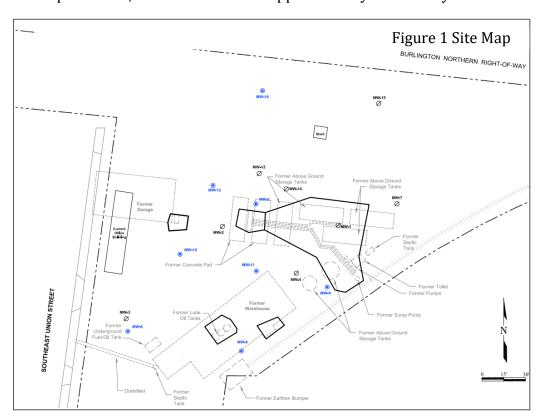
shows the areas of excavation (solid black lines), former structures (dotted gray lines) and monitoring well locations (blue dots).
