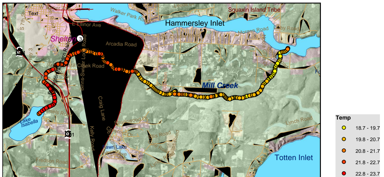
Figure 13. TIR survey of Mill Creek showing decreasing temperatures towards the mouth of the creek.
