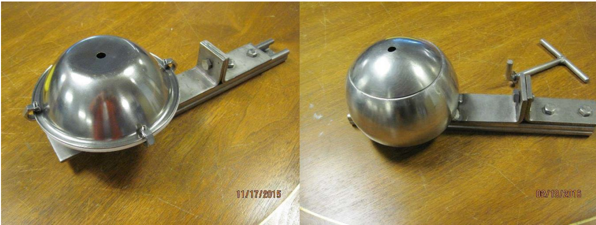
Photo 6 - Bowl-type trap prototype designed by City of Seattle (Seattle 2017)
