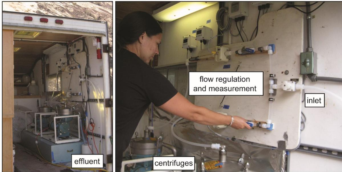
Figure 6. Centrifuge trailer (left) and the flow control board for each centrifuge (right).
