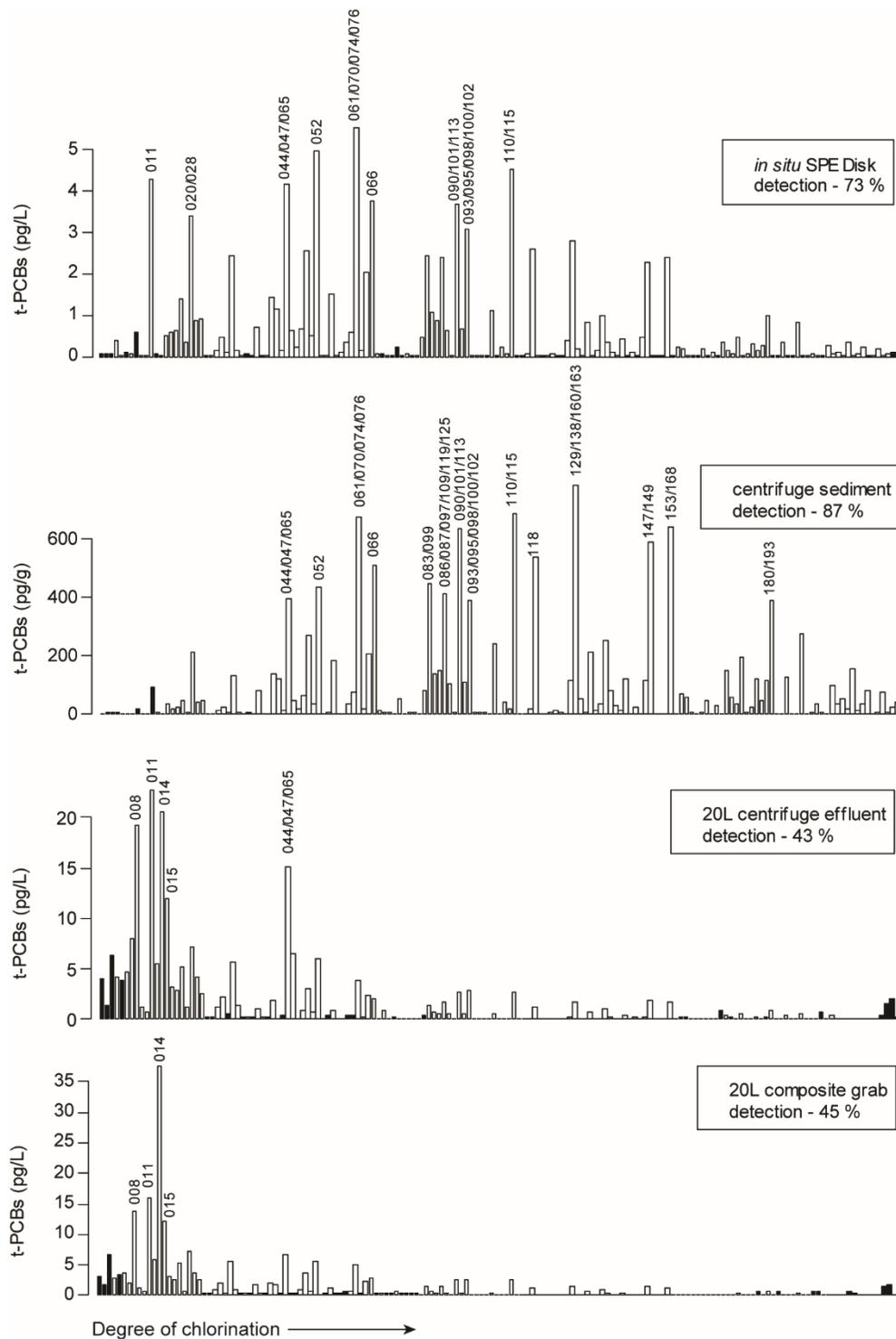
Figure 14. PCB congener profiles among the different sampling approaches from the Spokane River. Sampling method and frequency of detection are highlighted in the legend; the degree of chlorination increases from left to right; non-detect results are shown as black bars.
