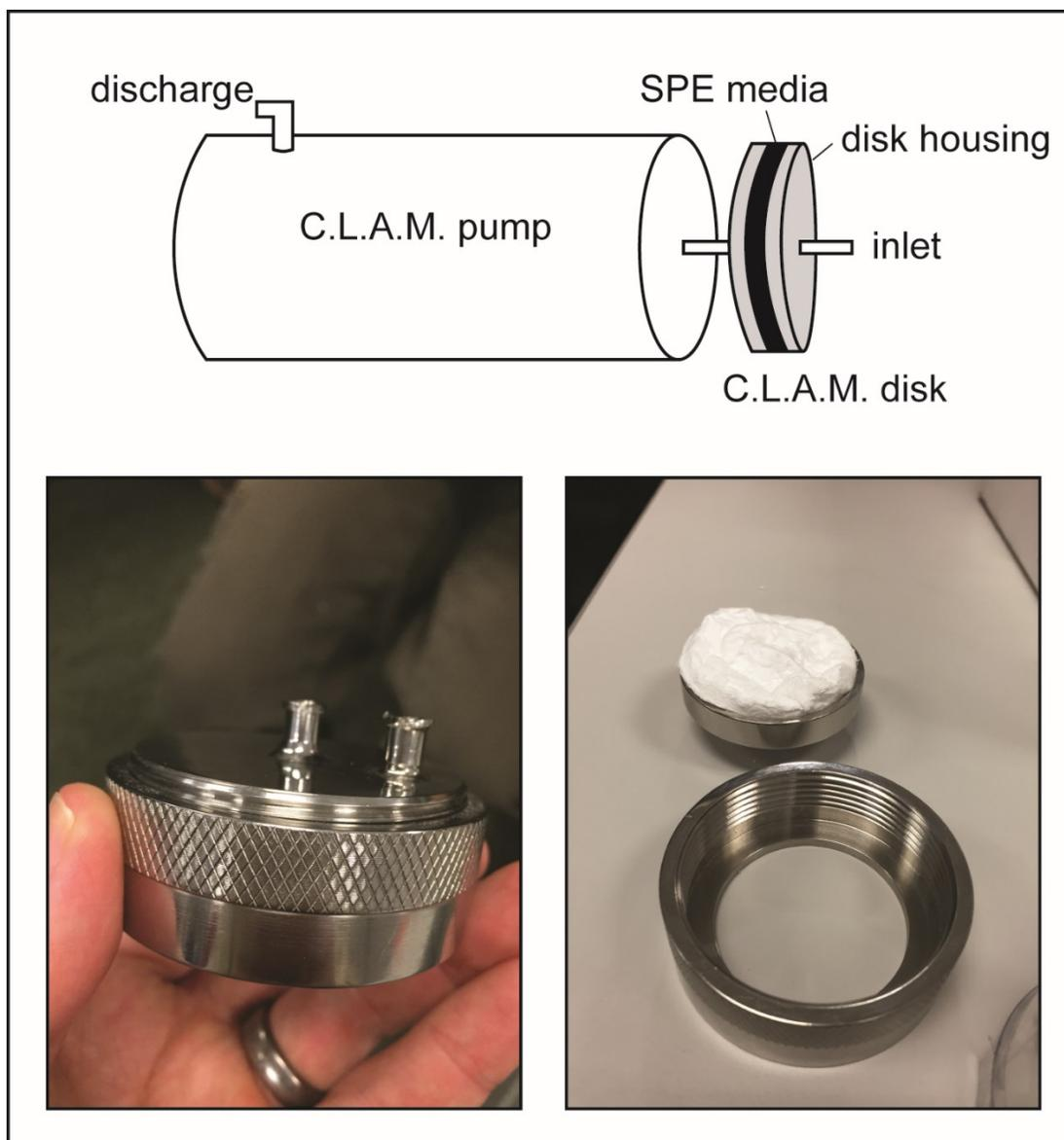
Figure 5. Parts of the CLAM sampler.
