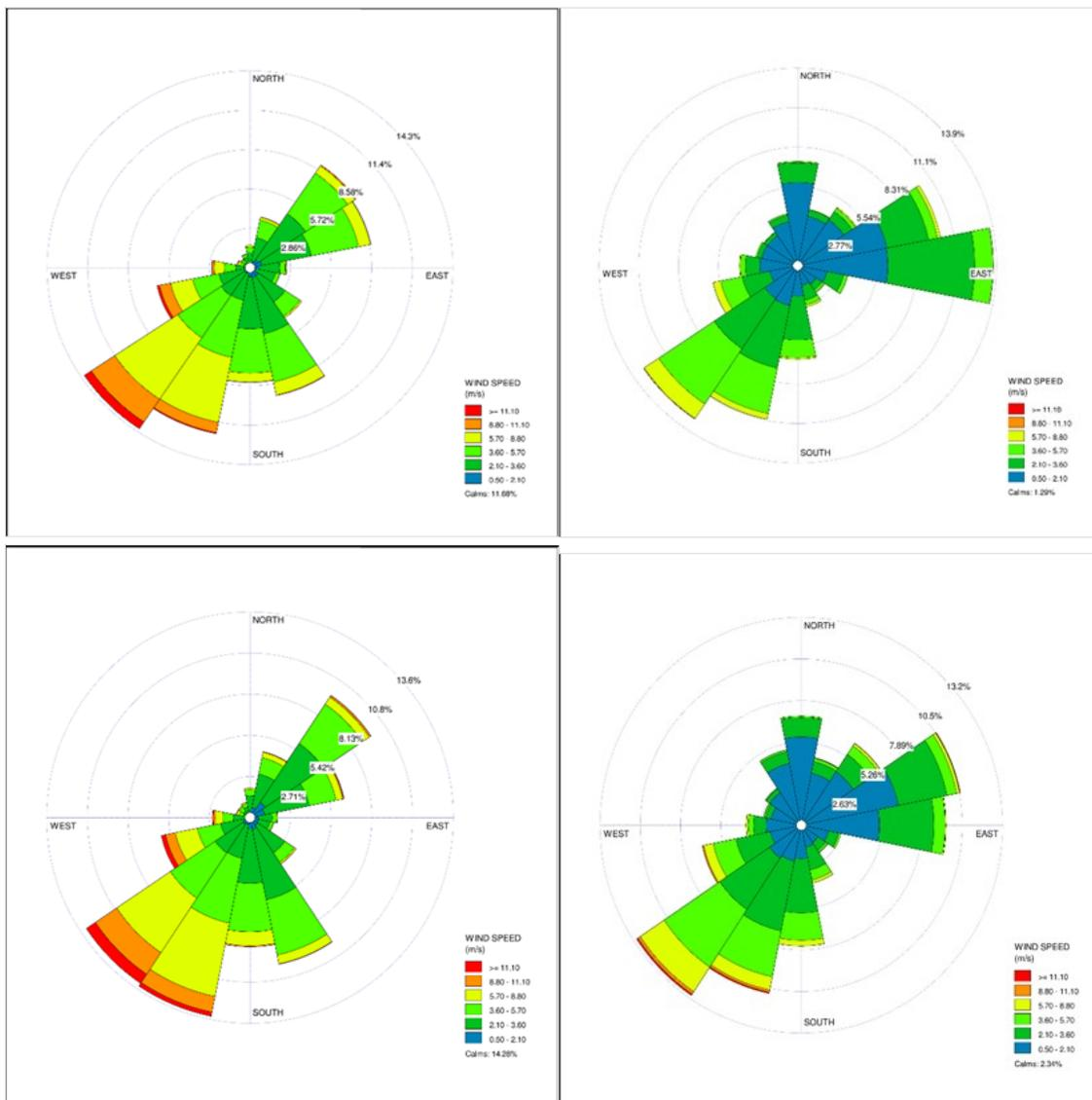
**Figure D3.** Wind rose plot of raw data (left panel) and pre-processed with 1-minute ASOS data (right panel) for January 2016 to June 2017 (upper) and January 2011 to January 2016 (lower), for the Spokane International Airport National Weather Service meteorological station.
