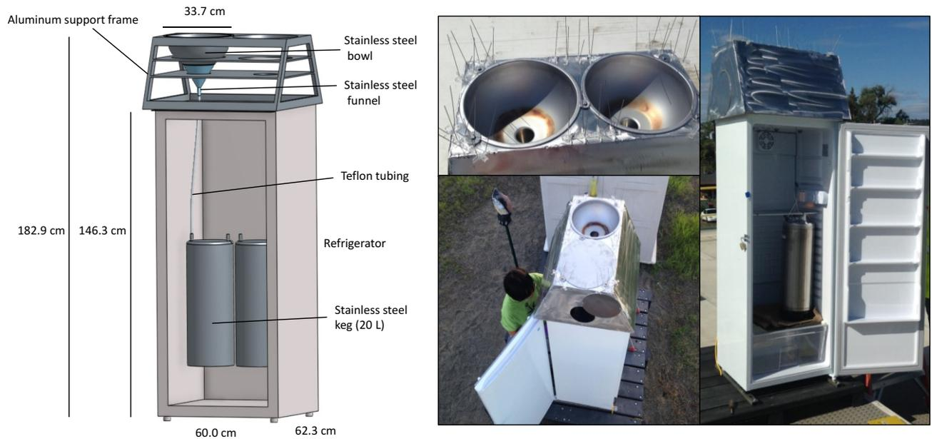
Figure 3. Schematic and photos of a bulk deposition sampler.
