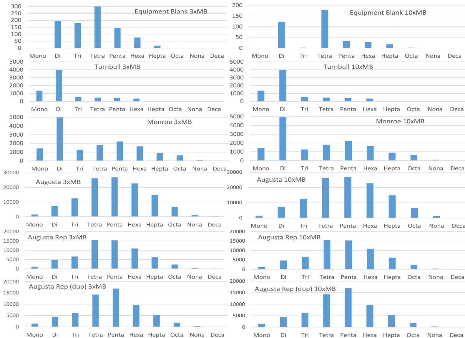
Figure B-2. Quarter 2 bulk deposition mass (pg) PCB homologues, censored at three and ten times the method blank (MB).
