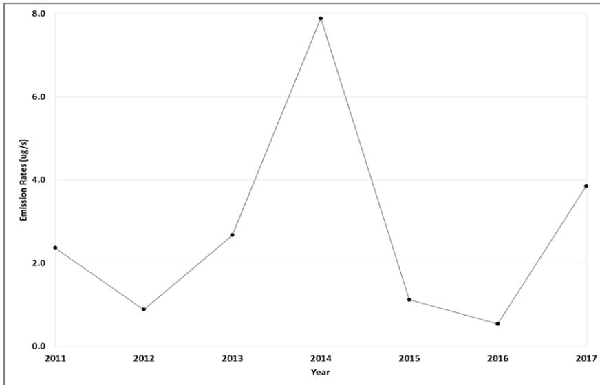
**Figure D4.** Spokane WTE Facility single-unit PCBs emission rates, estimated from measurement runs for 2011 through 2017 using equation 1.
