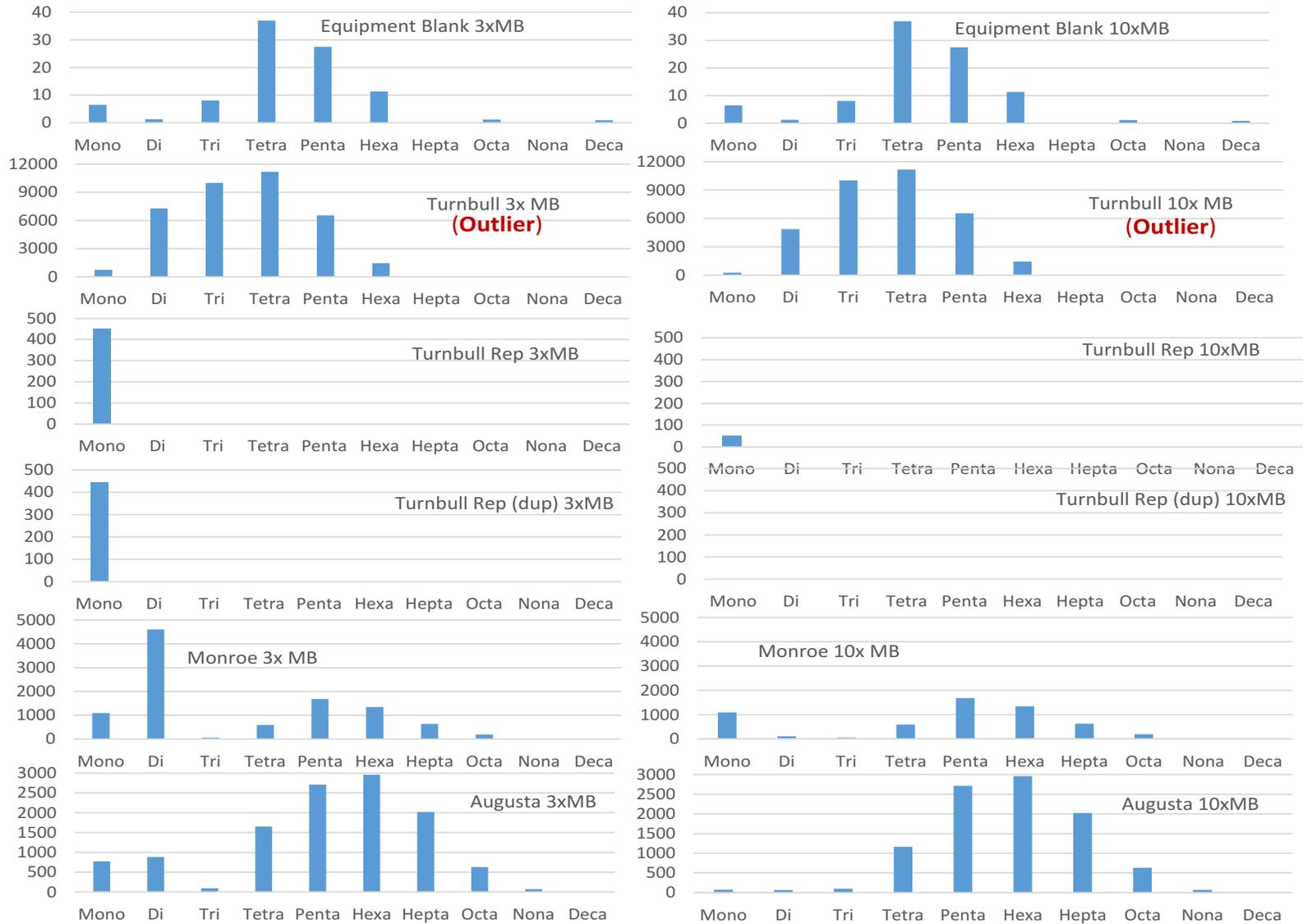
Figure B-4. Quarter 4 bulk deposition mass (pg) PCB homologues, censored at three and ten times the method blank (MB).
