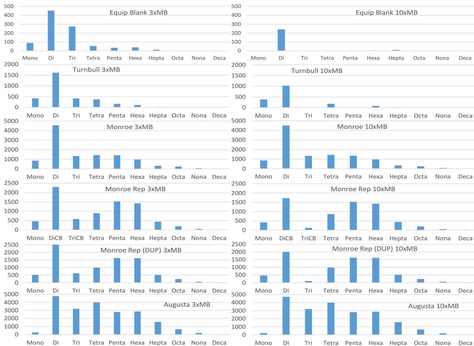
Figure B-1. Quarter 1 bulk deposition mass (pg) PCB homologues, censored at three and ten times the method blank (MB).
