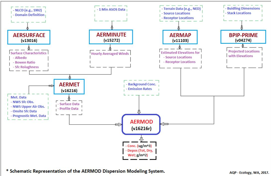
**Figure D2.** The AERMOD dispersion modeling system (with program versions) is depicted schematically, with the required input data for each program and their expected outputs.
