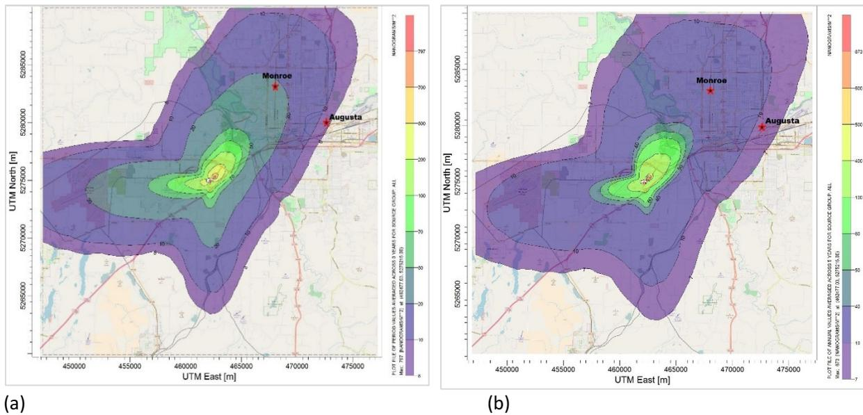
**Figure D6.** Modeled average annual total (bulk) deposition distribution from the Spokane WTE stack. (a) For May 11, 2016, to May 11, 2017, field measurement case study. (b) Regulatory 5-year modeling study period of January 2011 to December 2015. Coordinates are in UTM (m) and deposition is in nanograms per square meter ( $\text{ng}/\text{m}^2$ ).
