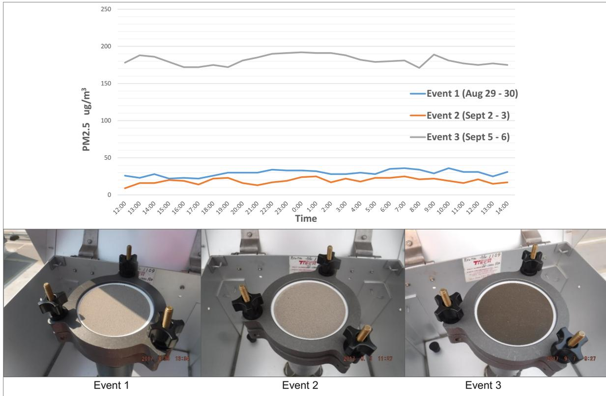
Figure 13. PM2.5 data (top) and photos of PUF filters after sampling wildfire smoke (bottom).
