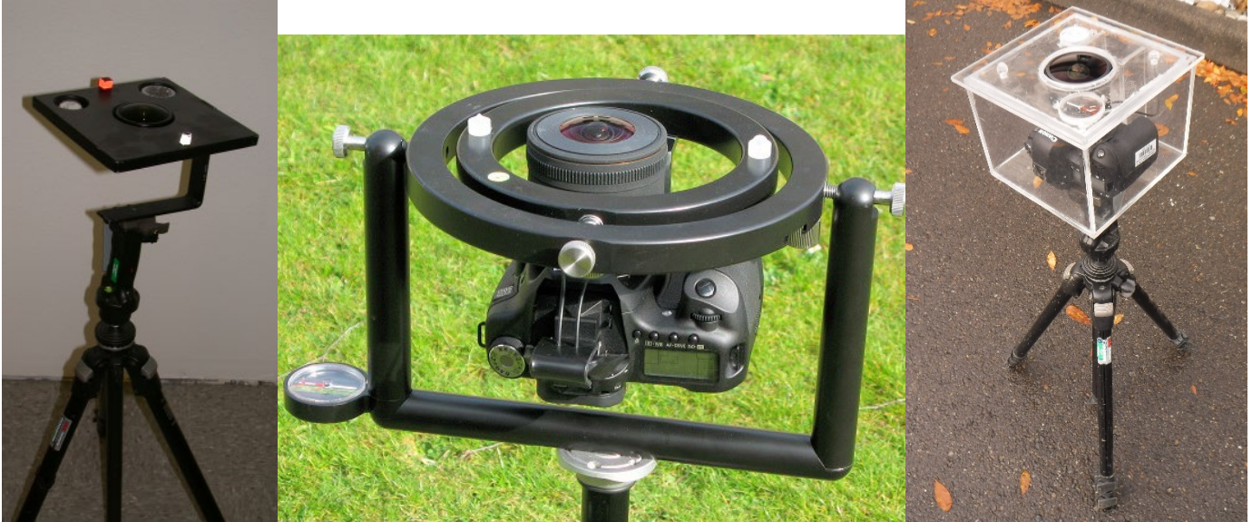
Figure 2: Left: Coolpix lens mount system used by Ecology; Center: Gimbal lens mounting device from Delta-T devices (SLM9). Right: EOS 6D lens mount system used by Ecology.
