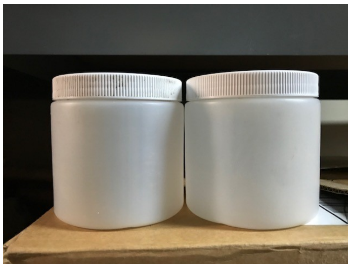
Figure 3. Sterile 16 ounce HDPE jars, one 'coarse jar' for epilithic, epidendric, or emergent epiphytic samples and one 'fines/macrophyte jar' for epipellic, epipsammic, or submerged epiphytic samples. See table 2 for details.
