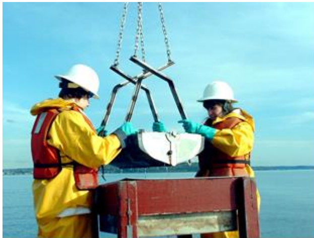
Figure 2. Marine Monitoring Unit staff landing a Van Veen sampler.
