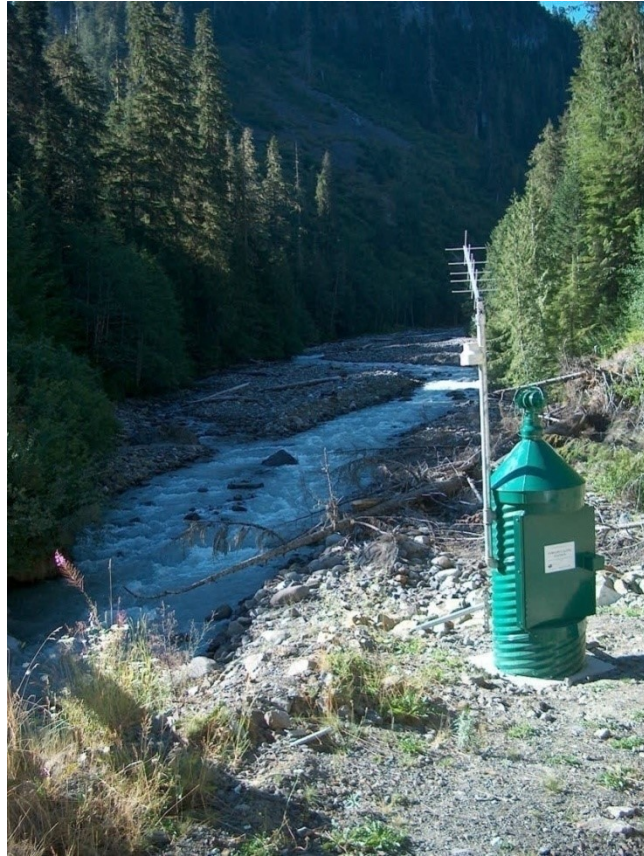
Figure 1 An example of a Fresh Water Monitoring Unit Flow Monitoring Station (Photo by Washington Dept. of Ecology)
