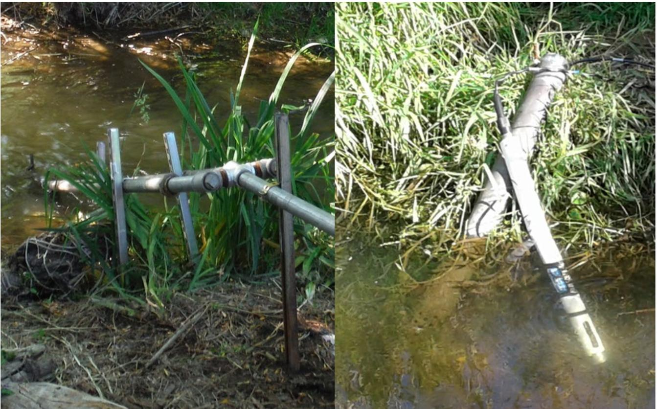
Figure 3. Examples of strut-channel (left) and simple rebar (right) bank-anchored installations.
