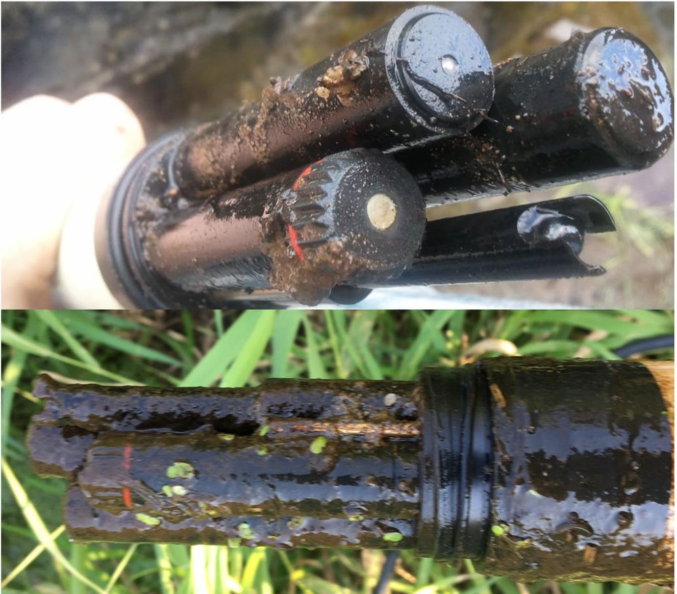
Figure 6. Sensor fouling due to sedimentation/debris accumulation (top) and eutrophic conditions (bottom).
