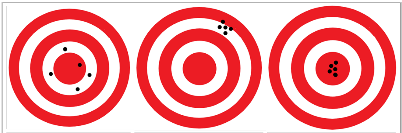
Figure 1. Illustration of accuracy vs. precision, as applied to Winkler and optical DO methods Additional text describing Figure 1:
