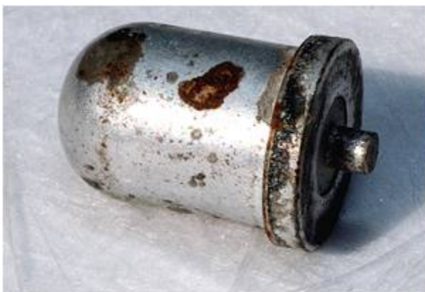
Mercury-containing ampule from an automotive mercury switch.
