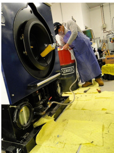
Figure 2. Pumping PERC from tanks. Photo by Stephen G. Whittaker, King County
