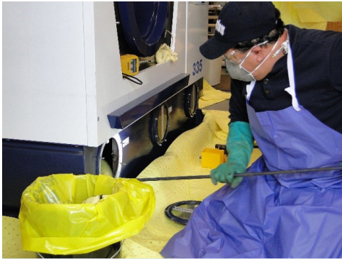
Worker prepares PERC machine to decommission. Photo Stephen G. Whittaker
