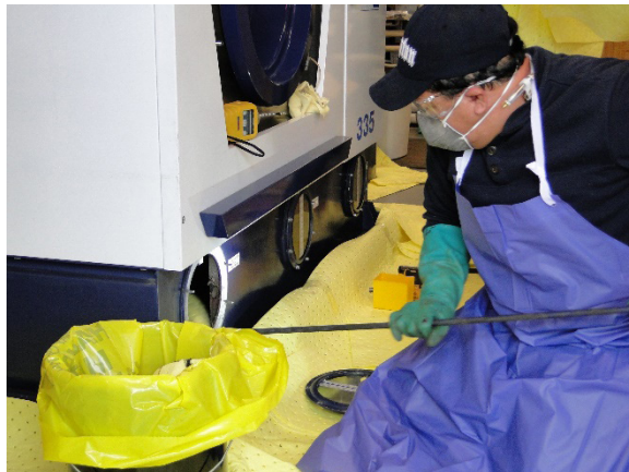
Figure 6. Place spent absorbent pads in a waste drum for proper disposal. Photo by Stephen G. Whittaker, King County
