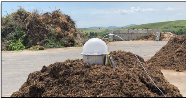
Figure 5: Photograph of flux isolation chamber at top of a 5% biochar pile
