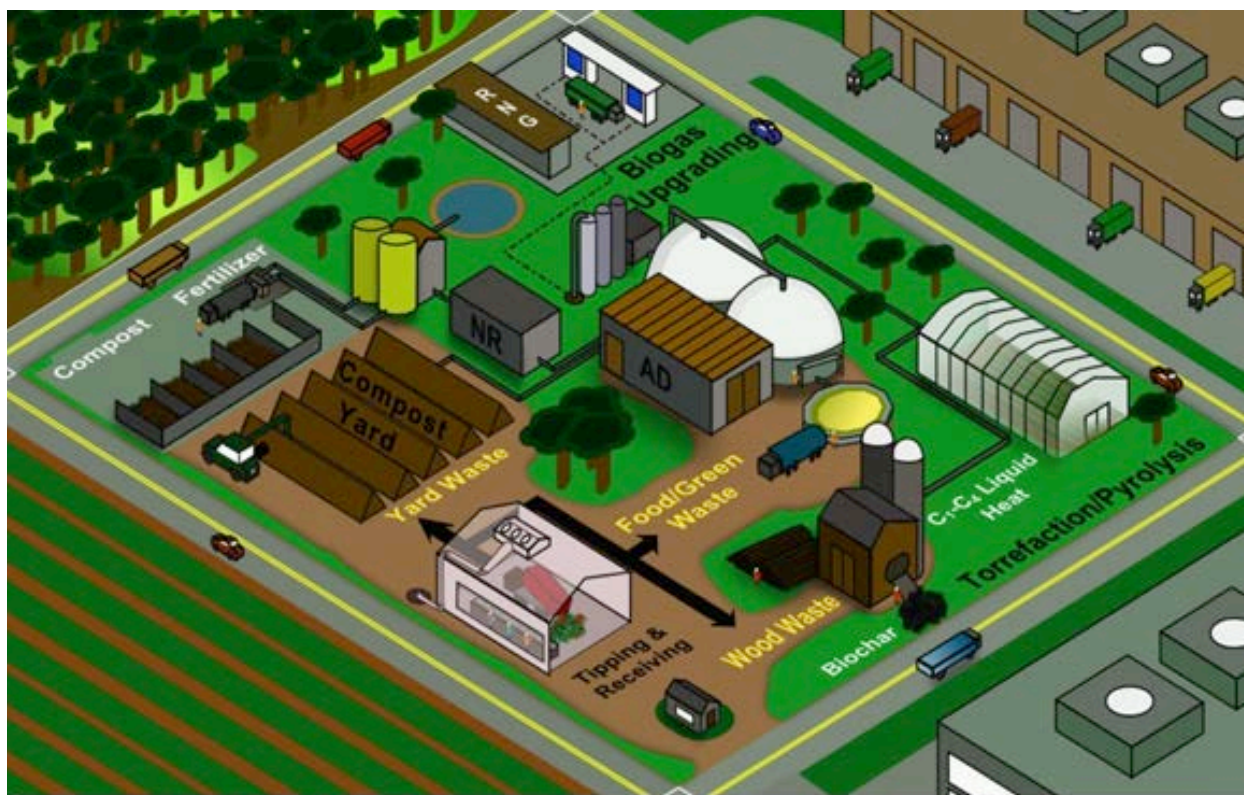
Figure ES.2: One possible realization of a municipal biorefinery. In this particular example, a core composting facility is transformed into a biorefinery through the addition of pyrolysis for treating a fraction of the wood wastes, and anaerobic digestion (AD) for treating food wastes. Nutrient recovery (NR) technologies and biogas upgrading to renewable natural gas (RNG) generate value-added products, while waste heat from pyrolysis is used for greenhouse production. Figure: Nick Kennedy
