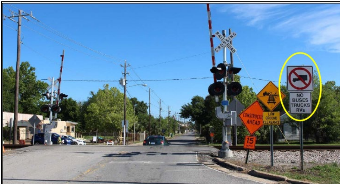
Figure 102: Low-Clearance High-Profile Crossing with Prohibition Sign in Biloxi, Mississippi 429
