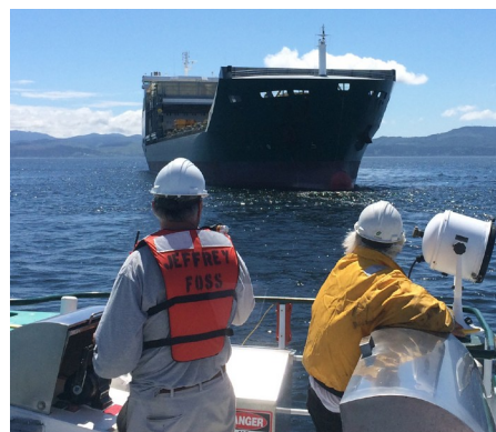
ERTV passing a tow line to a cargo ship that has lost propulsion.
