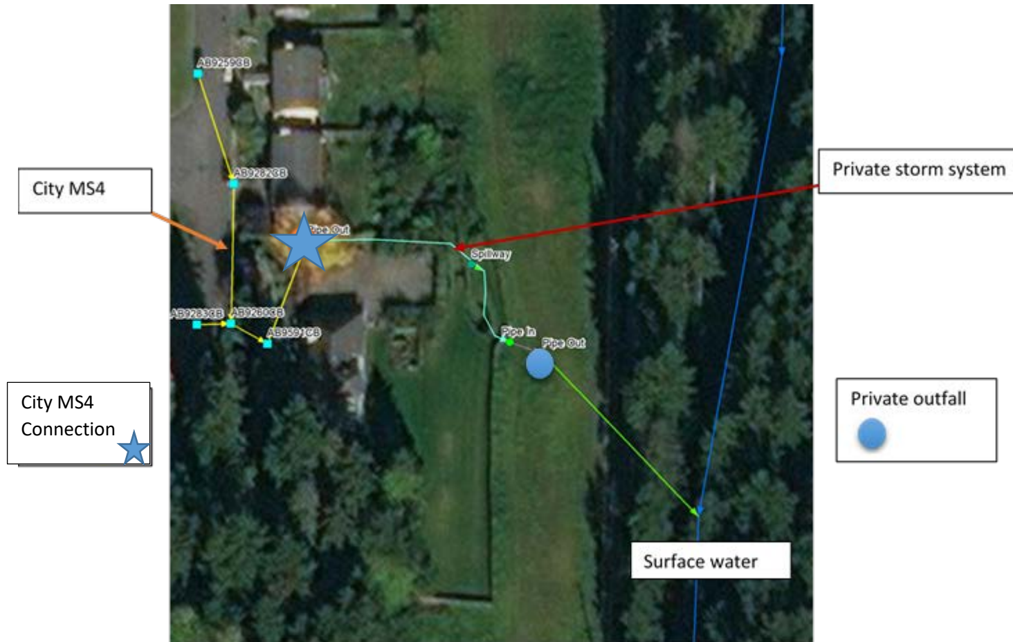
Figure 6 - Municipal System to Private Stormwater System
