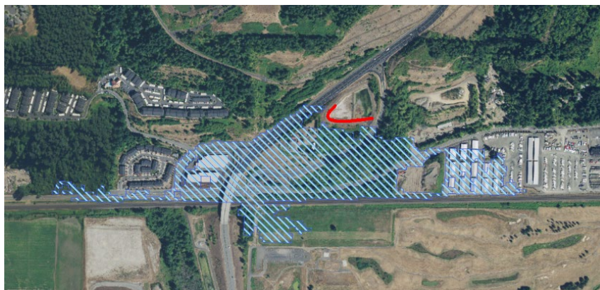
Inundated area (shown in blue) from a modelled dam breach (dam shown in red) in Pierce County, WA.
