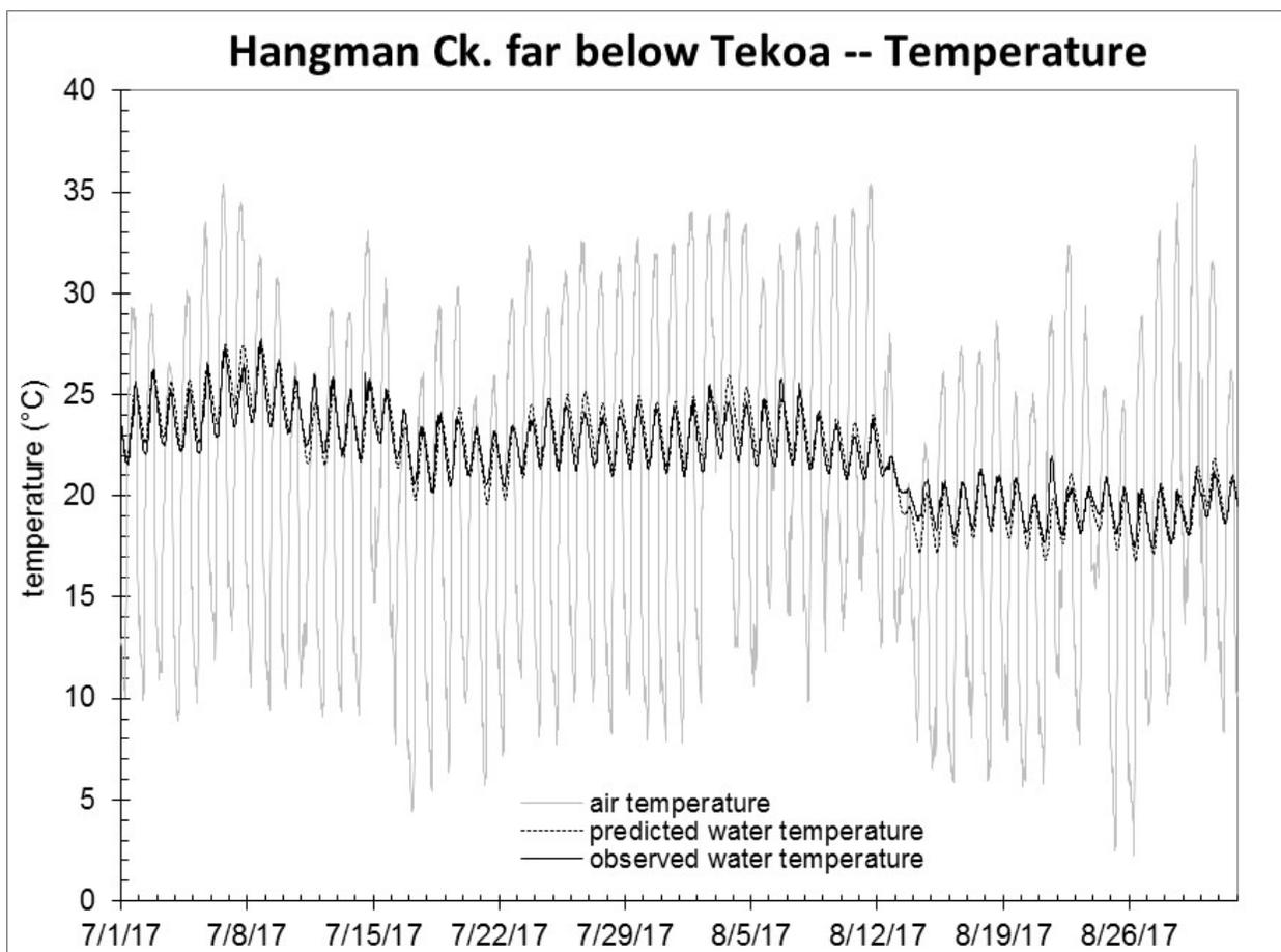
Figure 16. rTemp predicted and observed water temperatures
