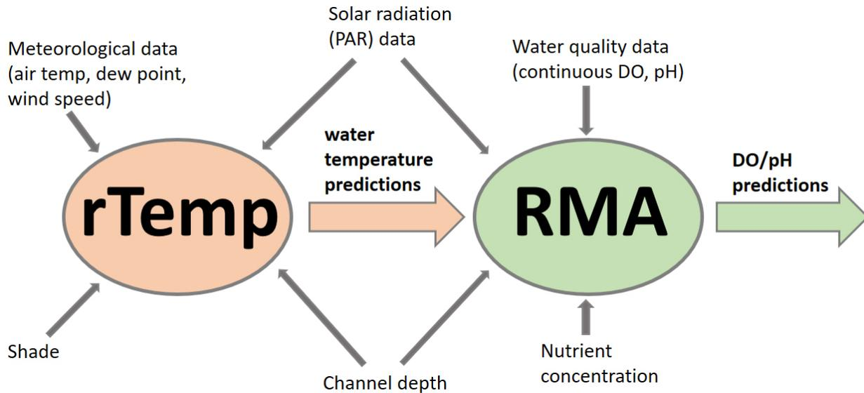
**Figure 15. Conceptual diagram showing linkage of rTemp and RMA water quality models.**
