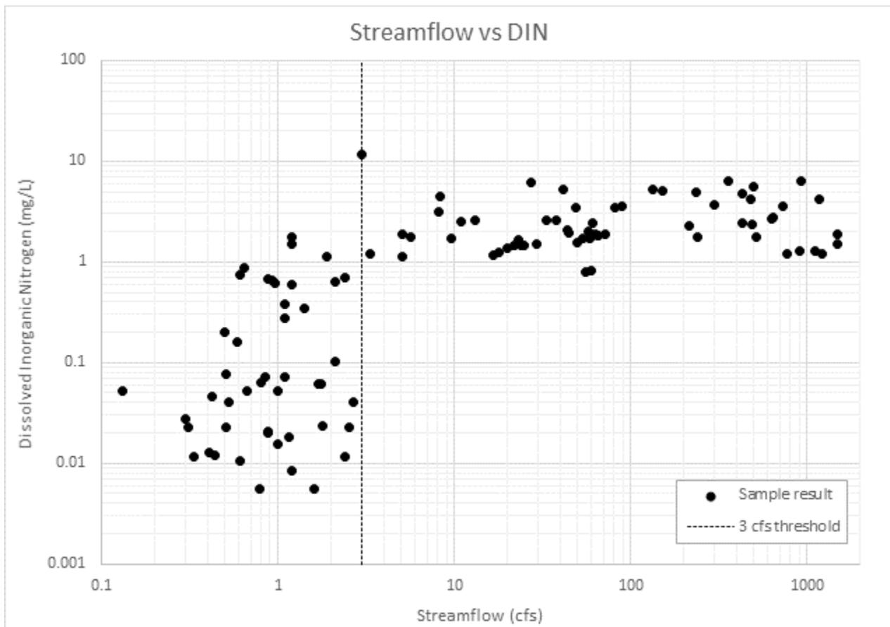
Figure E-1. The relationship between streamflow and dissolved inorganic nitrogen (DIN) in upper Hangman Creek during 2017 and 2018.
