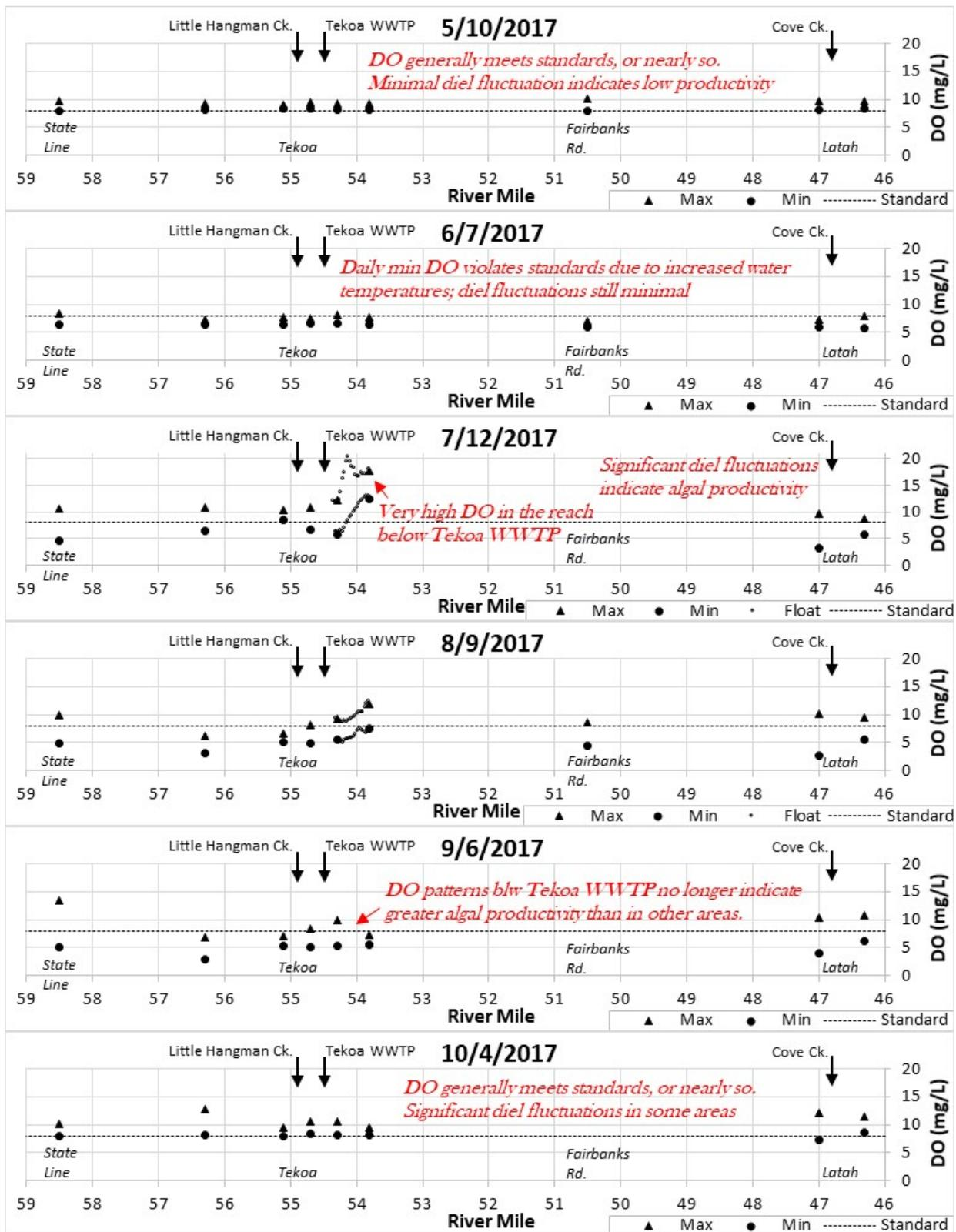
Figure 6. Daily maximum and minimum dissolved oxygen (DO) in upper Hangman Creek.
