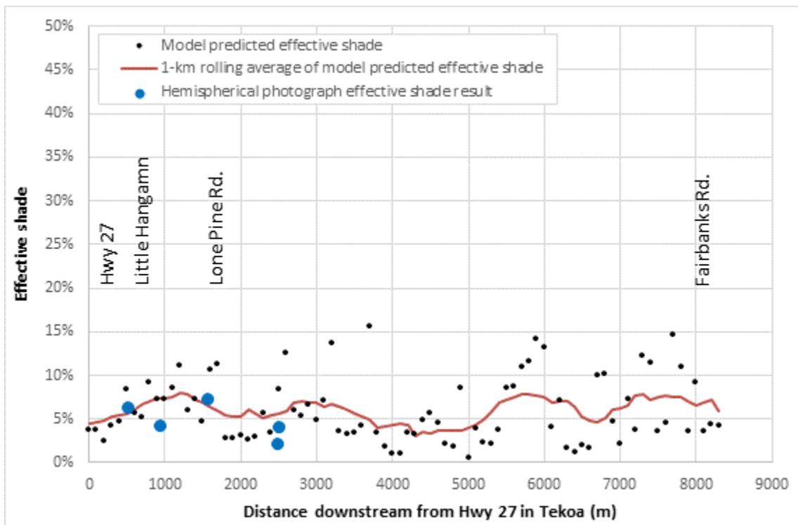
Figure D-2. Modeled and hemispherical photo calculated effective shade.
