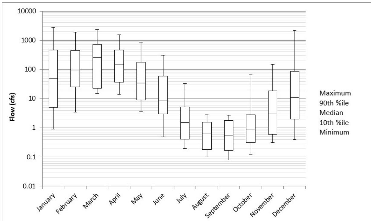
**Figure 2. USGS stream-gage monthly flow statistics between 2007 and 2019 for Hangman Creek at state line (Gage ID 12422990).**
