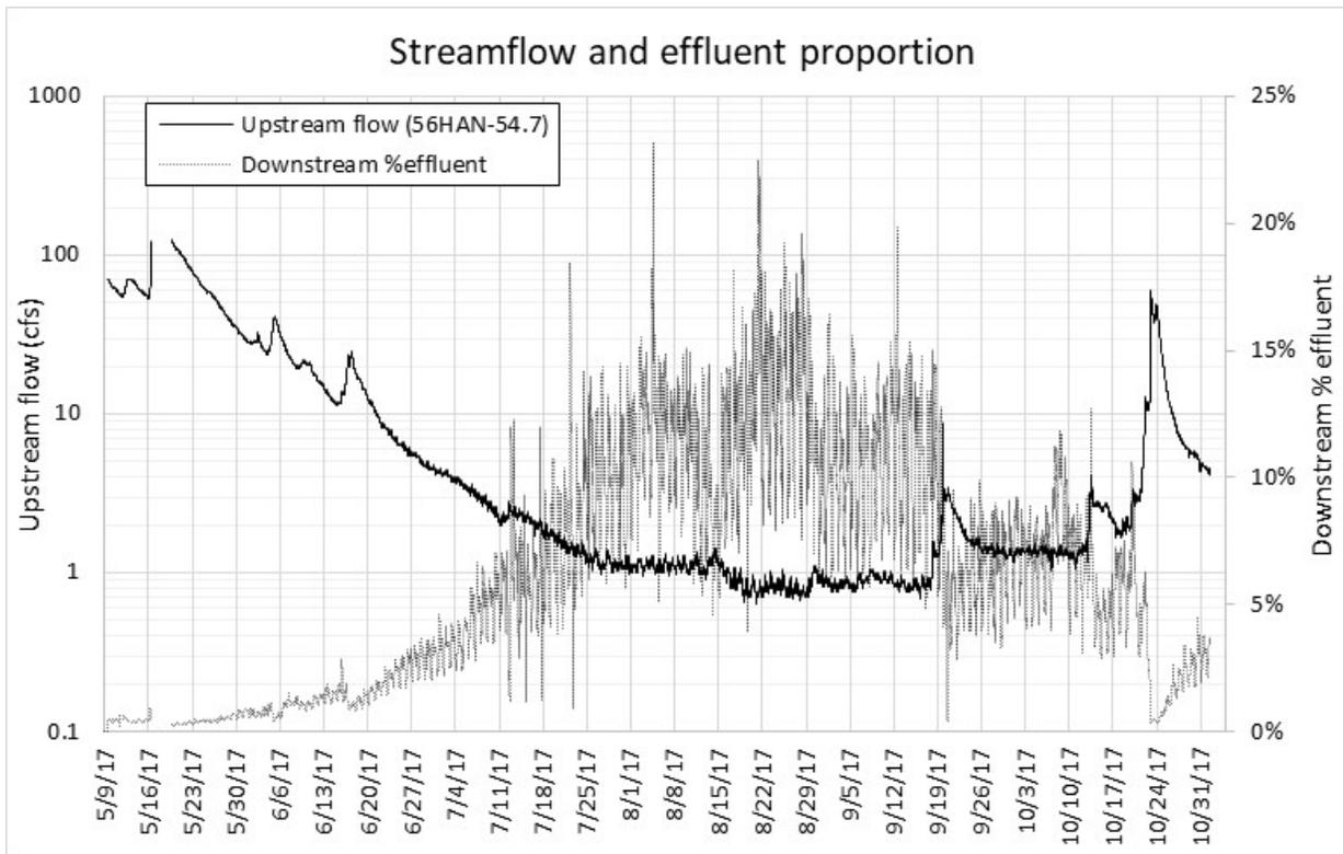
Figure 13. Streamflow upstream of Tekoa WWTP, and downstream effluent proportion.
