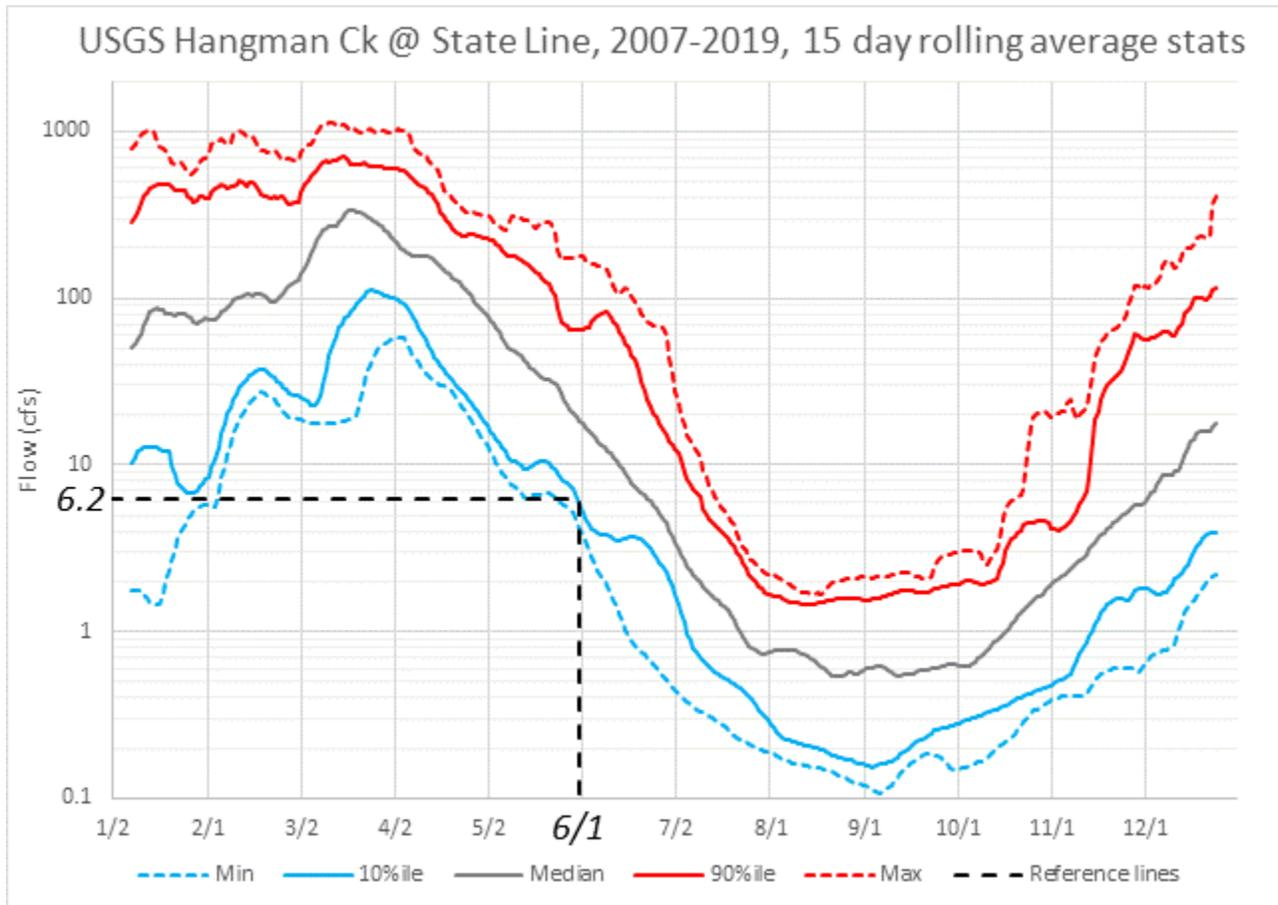
**Figure E-3. Flow statistics for USGS Hangman Creek at State Line, showing derivation of June 1 seasonal window start date.**
