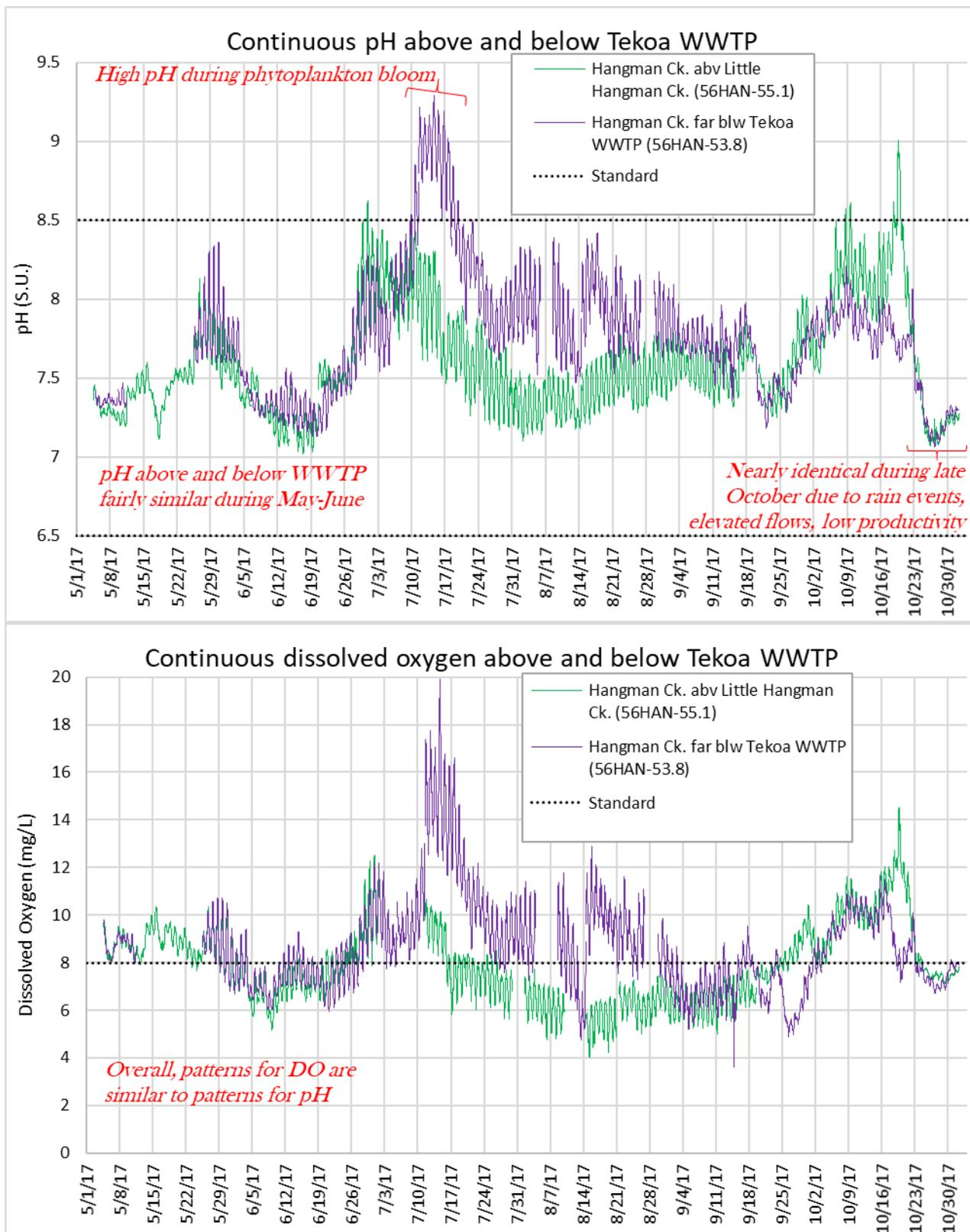
**Figure 7. Continuous pH and DO in Hangman Creek above and below Tekoa WWTP.**
