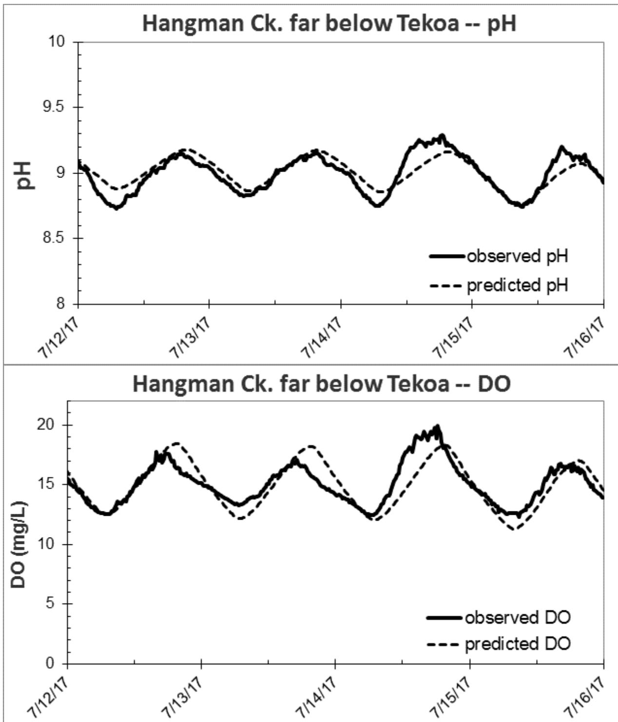
Figure 17. RMA predicted and observed DO and pH
