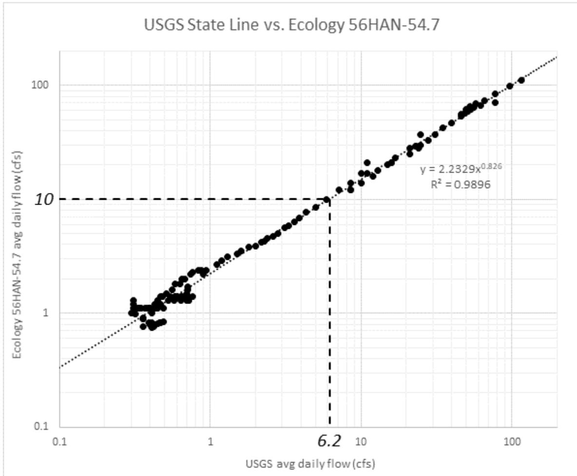
**Figure E-2. Comparison of gaged streamflows at 56HAN-54.7 (Hangman Ck. at Rodeo Grounds) and USGS Hangman Ck. at State Line.**
