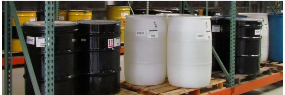
Figure 1: Drums containing dangerous waste, properly labeled and stored safely while waiting for disposal or treatment by generator.
