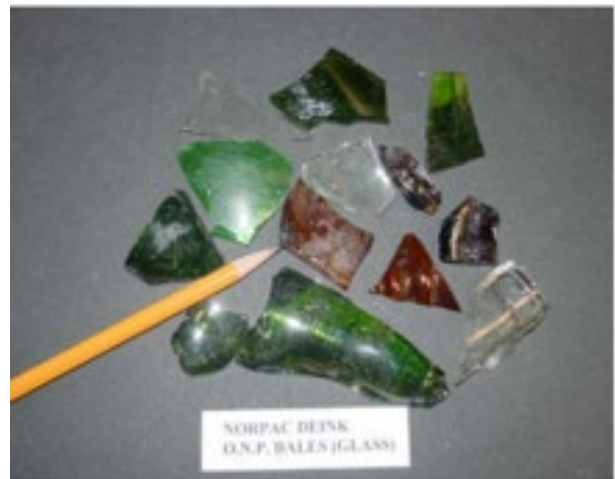
Figure 6: Glass collected in commingled recycling programs can end up at paper mills and seriously damage papermaking equipment. This 2009 photo shows glass that was in a paper bale and rejected in the pulping process at NORPAC.
