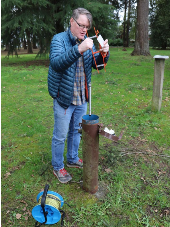
John Pearch, Southwest Regional Well Construction Inspector, measures the static water level in a well. This activity is part of the Well Drilling Management Program.
