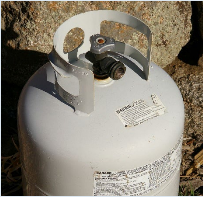
Figure 1: Propane tanks are empty when the pressure inside is equal to or nearly equal to atmospheric pressure.
