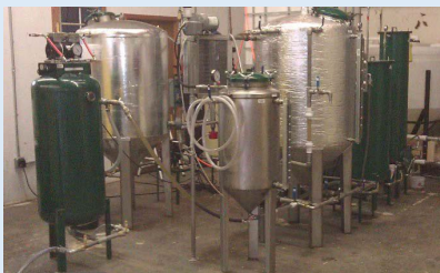
Figure 3: You may treat dangerous wastewater in a totally enclosed treatment unit.
