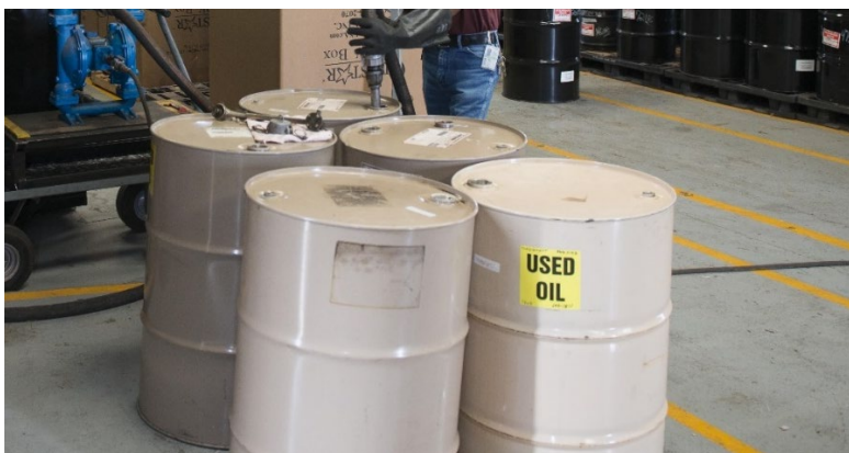
Figure 14: Clearly mark used oil containers. Store them in an area with an impermeable floor.
