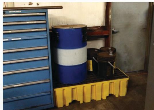
*After: Containers moved to the other side of the door and placed on secondary containment pallet. Now, if there's a spill or overflow, any extra materials will be captured by the secondary containment pallet.*
