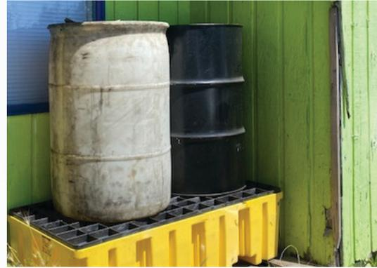
*After: With secondary containment, even if there is a spill or overflow, any spilled materials will be captured with the secondary containment pallet and can be properly managed.*
