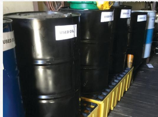
*After: Drums of used oil placed on secondary containment pallets and moved inside under cover. This is a cleaner and safer way to store used oil.*
