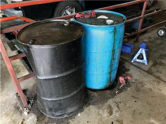
*Before: The area lacked secondary containment. These drums were located next to stairs leading to the pit below. Spills in this area would be extra difficult to clean up.*
