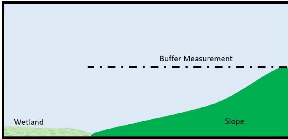
**Figure 6C-2. Measuring buffer widths on slopes.**
