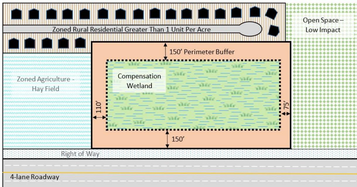
**Figure 6C-3. Variable width perimeter buffer**
