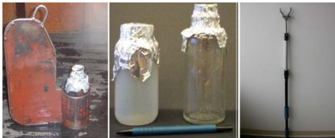
Figure 3. Bacteria water sampling equipment and sample bottles.
