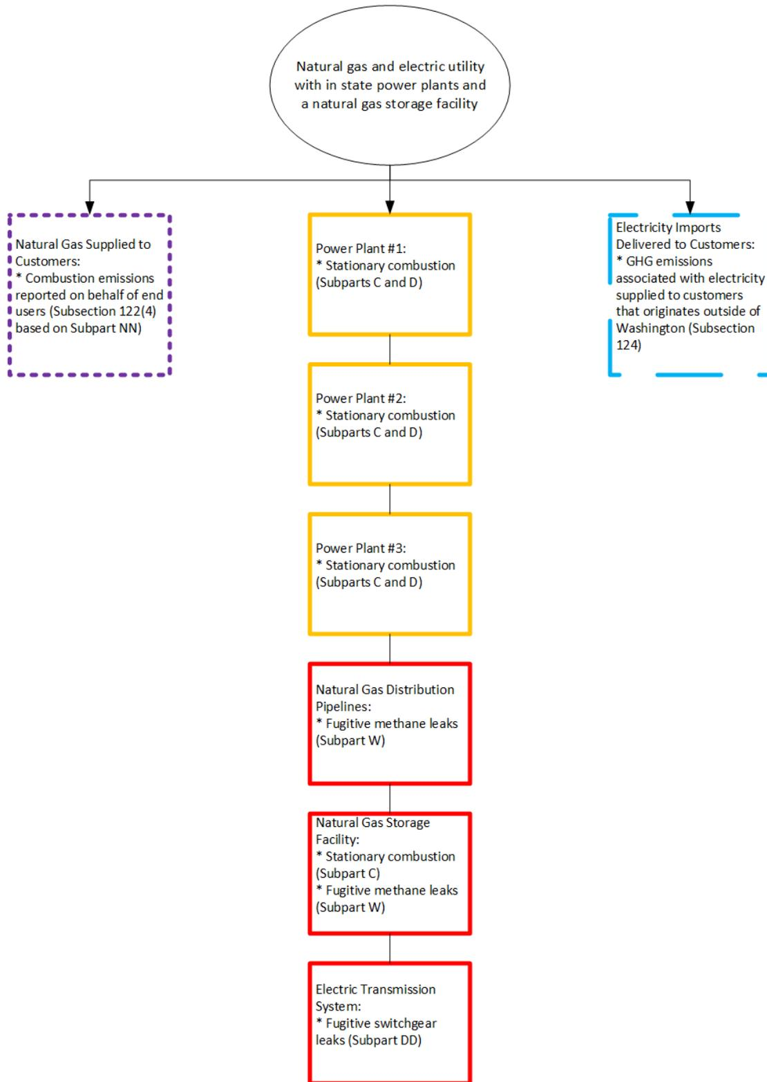
Figure 1: Example of a natural gas and electric utility with in-state power plants and a natural gas storage facility.
