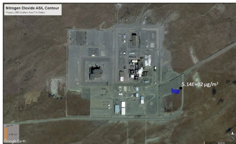
Figure 3: Modeled NO 2 greater-than-ASIL impact area near Southern Area Fire Station Emergency Generator
