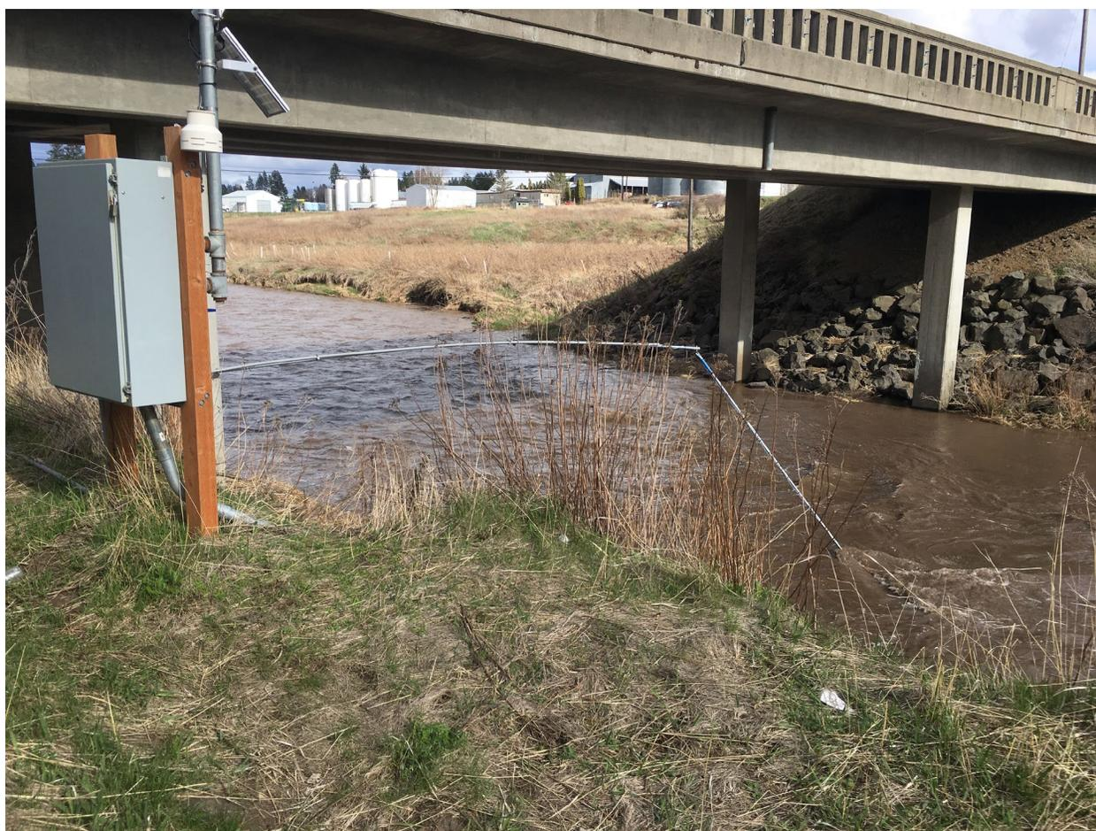
**Figure 8. Gage station at Rock Ck. at Hwy 27 (56ROC-13.0), with turbidity sensor mounted at the end of swing arm.**
