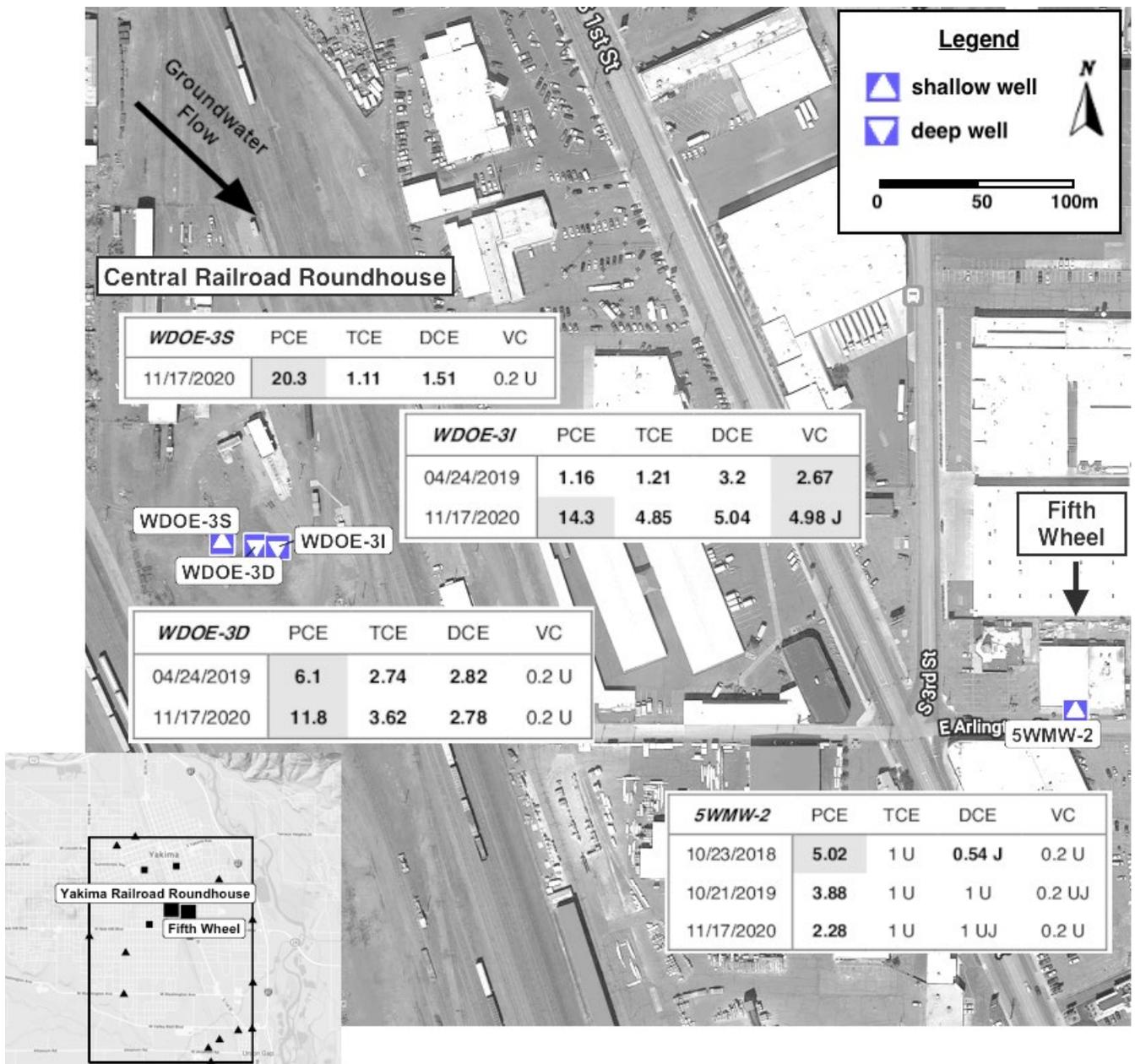
**Figure 6. Washington Central Railroad Roundhouse and Fifth Wheel Truck Repair Well Locations and cVOC Results (ug/L), 2018-2020.**
