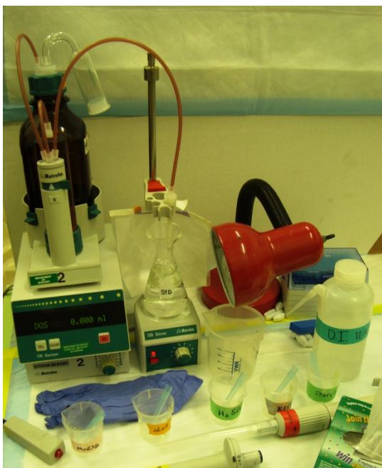
Figure 1 Dosimat with DO flask on stir plate, beakers for each reagent, pipettes, deionized water in squeeze bottle, desk lamp, laboratory gloves, and Kimwipes.
