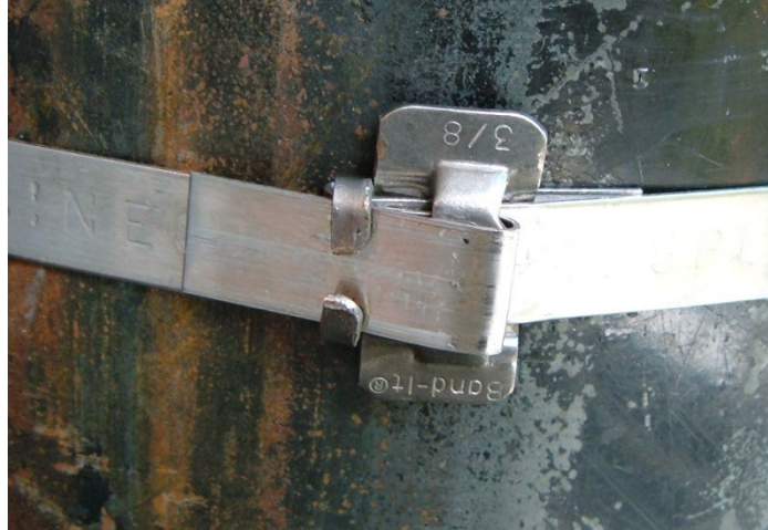
Figure 11. Folding the clamp tangs
