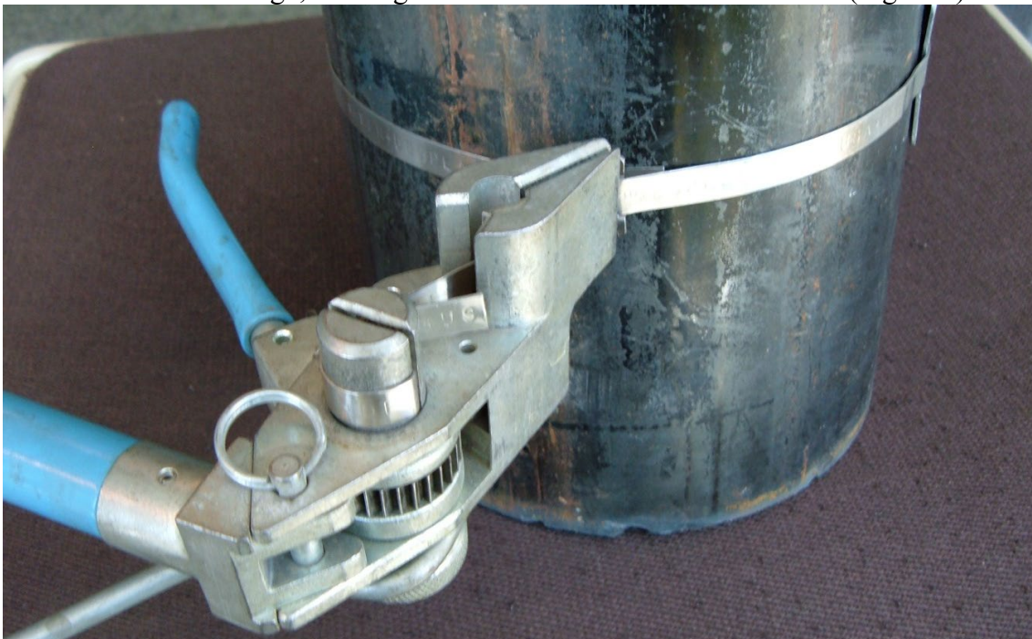
Figure 8. Rolling the banding tool
