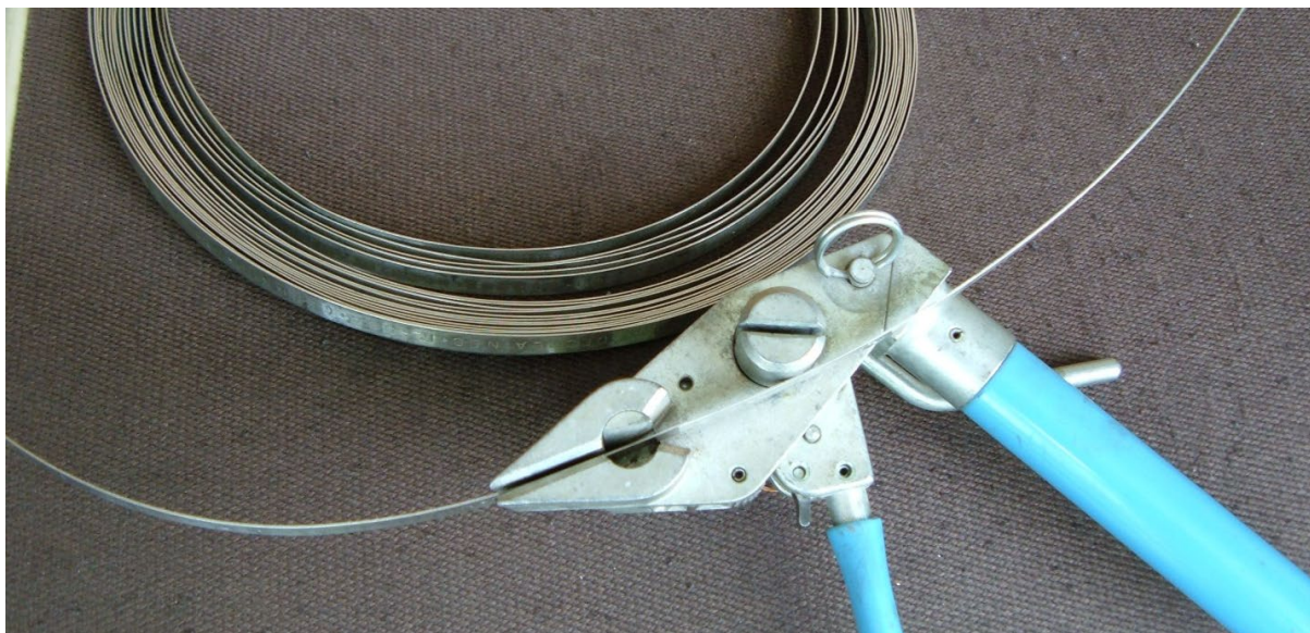
Figure 2. Cutting the banding to length
