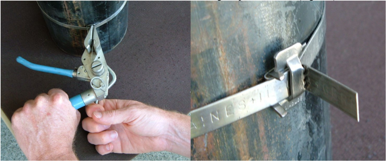
Figure 9. Cutting the band
