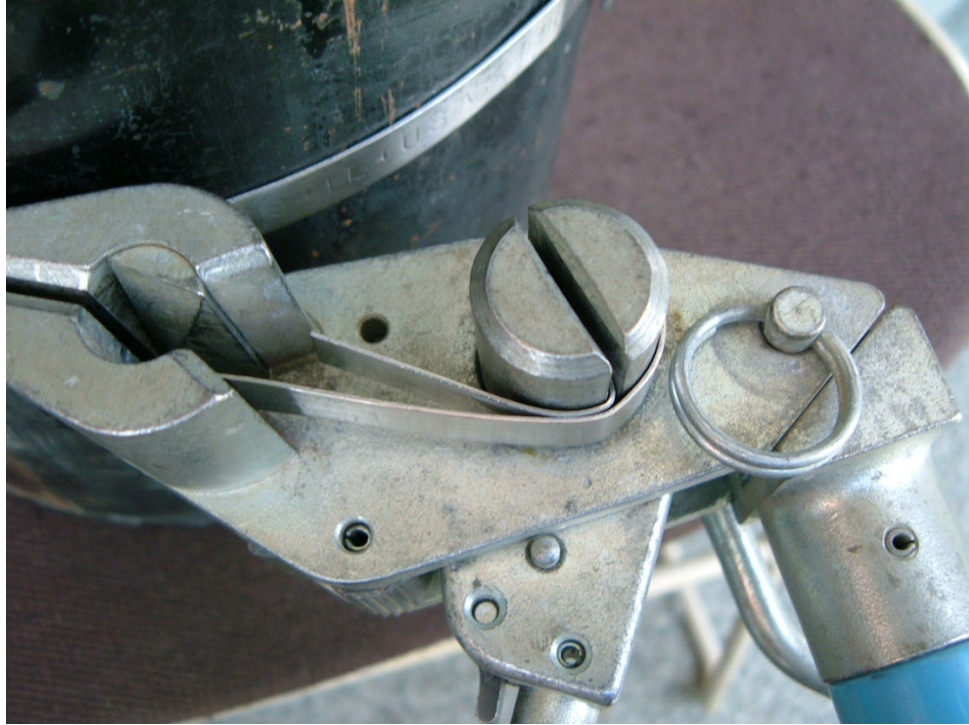
Figure 7. Tightening the band
