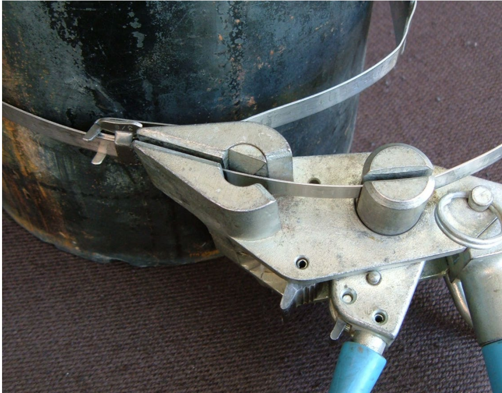
Figure 6. Threading the banding tool
