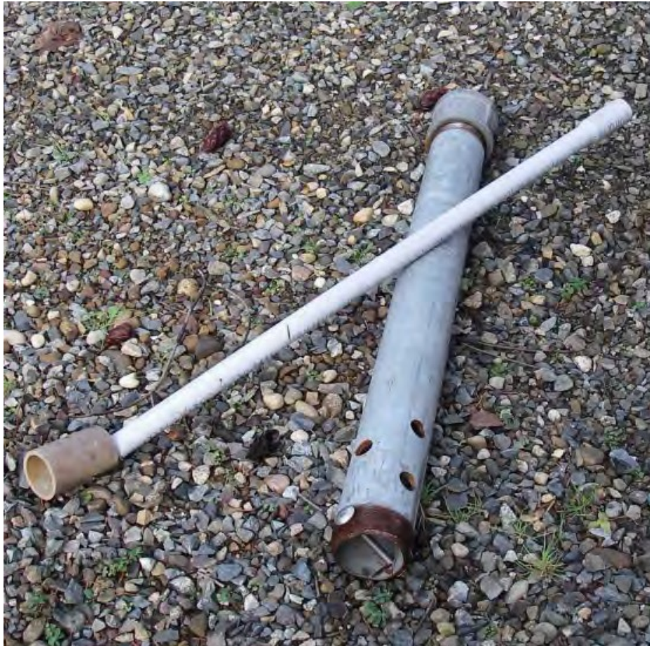
Figure 3: Deployment method using a length of PVC pipe
