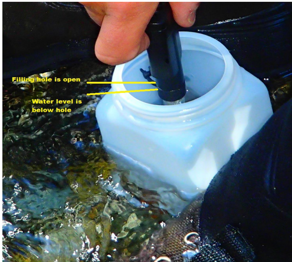
Figure 4: Measuring pH at equilibrated temperature and outside of streamflow.
