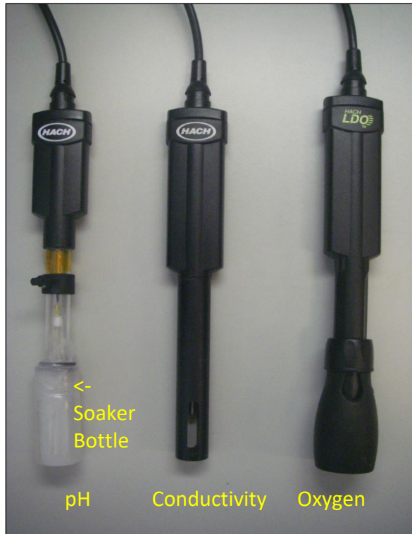
Figure 2: PHC28101 IntelliCAL pH Ultra Electrode, CDC401 IntelliCAL Standard Conductivity Probe, and LDO101 IntelliCAL Standard Dissolved Oxygen Probe.
