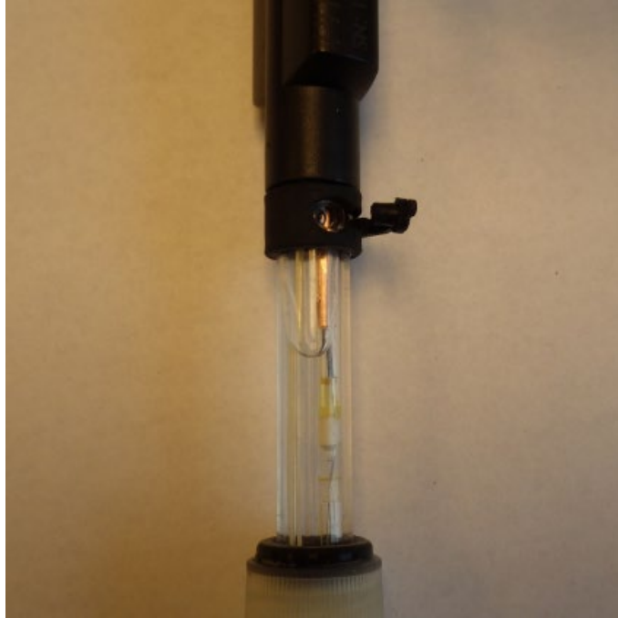
Figure 3: Close-up of electrolyte filling hole on pH probe
