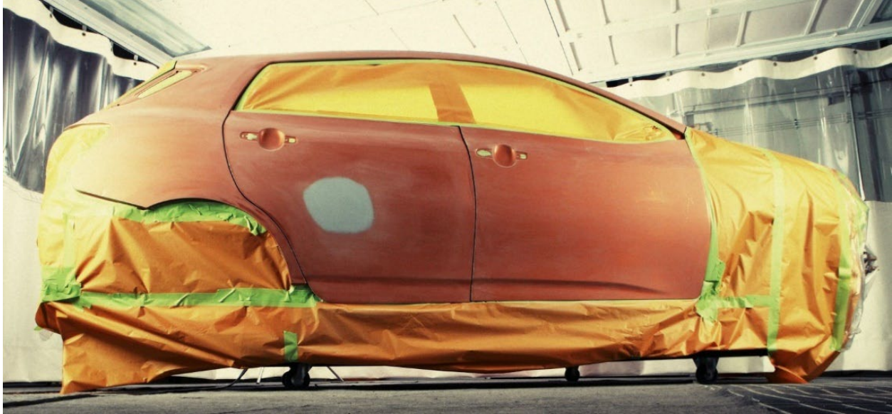
Figure 1: Used masking tape, overspray paper, paint filters, and more may be dangerous waste.
