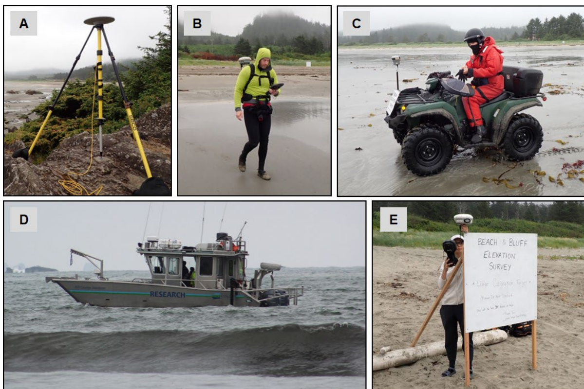
Figure 12. Topo-bathymetric data collection techniques. A) GNSS Base station. B) Topographic data collection using GNSS mounted on backpacks. C) Topographic surface mapping using a GNSS mounted on an ATV. D) R/V George Davidson collecting MBES in the nearshore. E) Lidar target being surveyed.
