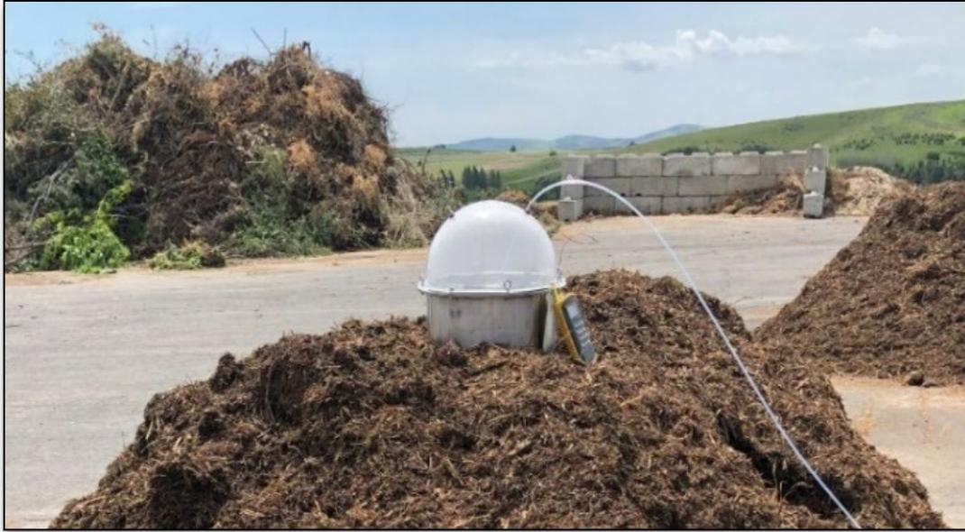
Figure 8: Photograph of flux isolation chamber at top of a 5% biochar pile.
