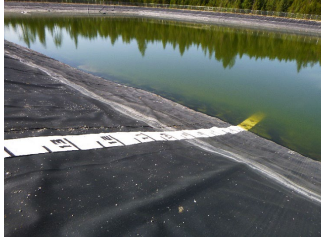
Example 4. Pond liner mounted staff gauge
