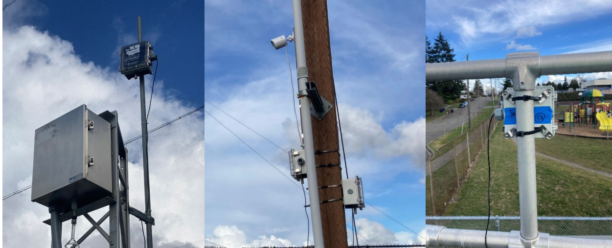
Figure 10. Pictures of SensWA mounted with high-strength zip ties.
