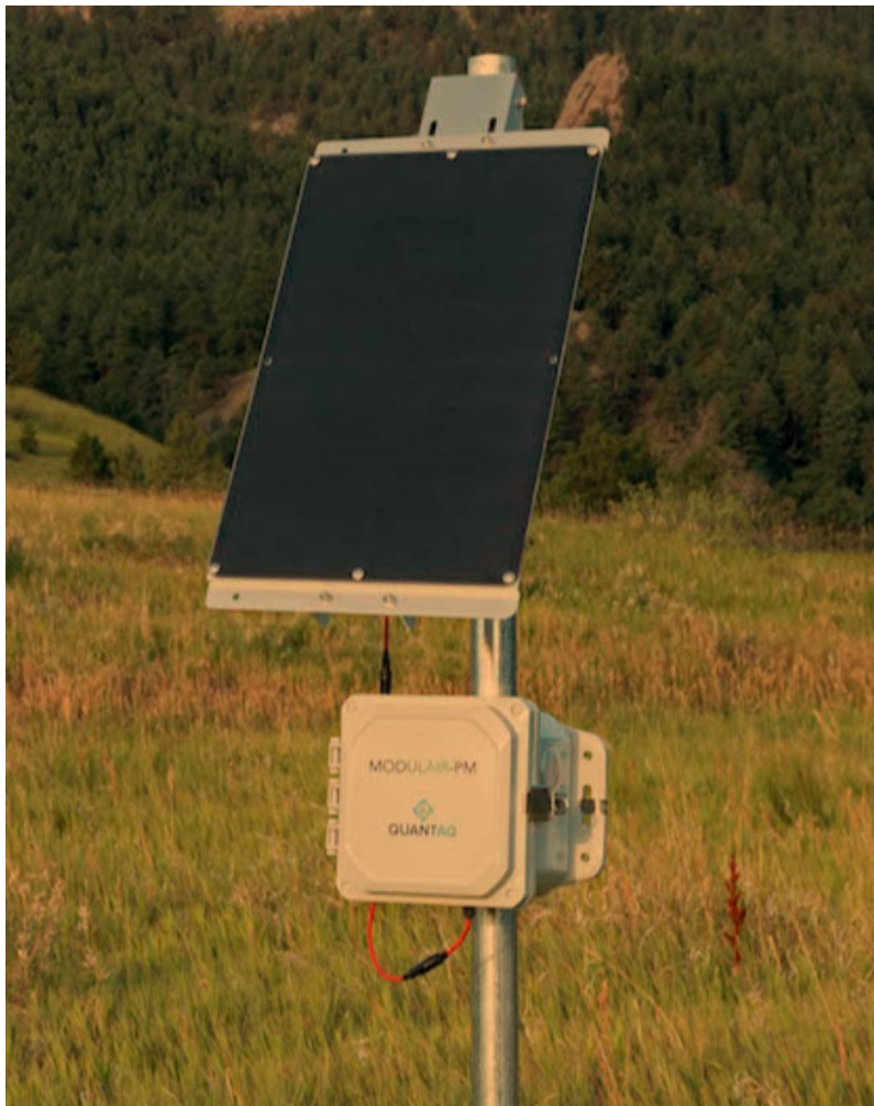
Figure 11. Picture of the MODULAIR-PM PM sensor, with optional solar panel power, mounted on a pole for ambient monitoring.
