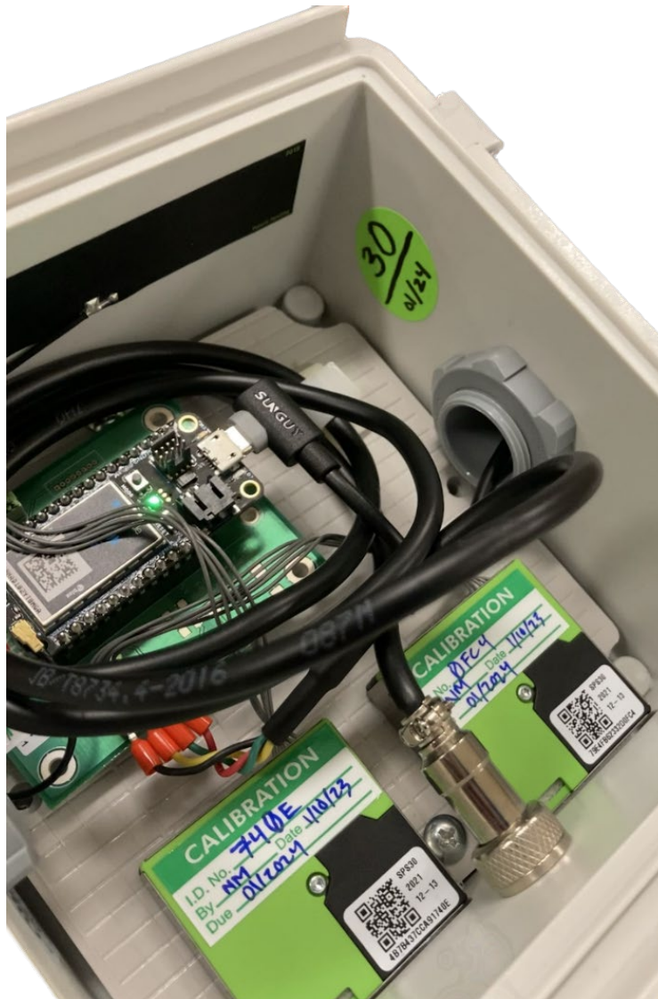
Figure 8. Ecology SensWA PM sensor internal components.
