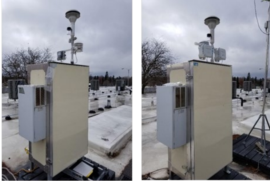
Figure 1. One SensWA PM 2.5 sensor collocated with a BAM PM 2.5 (left) and two QuantAQ MODULAIR-PM PM 10 sensors collocated with a BAM PM 10 (right) at the Spokane – E. Broadway Ave. monitoring site.
