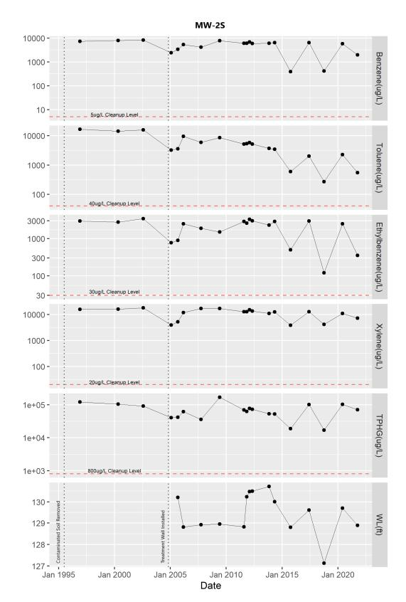
Figure A2. Contaminant concentrations ( $\mu g/L$ , log scale) and groundwater elevations (ft) for well MW-2S, November 1993 to October 2021.
