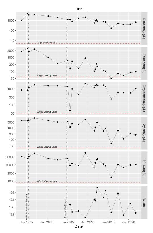
Figure A1. Contaminant concentrations (µg/L, log scale) and groundwater elevations (ft) for well D11, November 1993 to October 2021. Open circles indicate analyte was not detected and are plotted at one-half the reporting limit.
