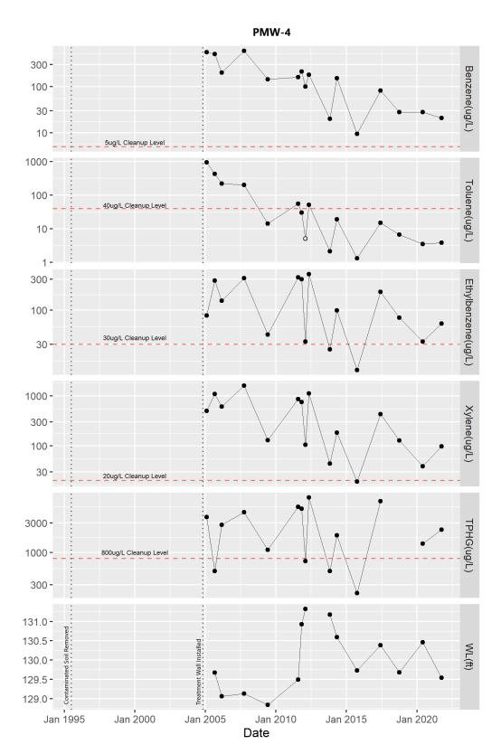
Figure A4. Contaminant concentrations (μg/L, log scale) and groundwater elevations (ft) for well PMW-4, November 1993 to October 2021. Open circles indicate analyte was not detected and are plotted at one-half the reporting limit.
