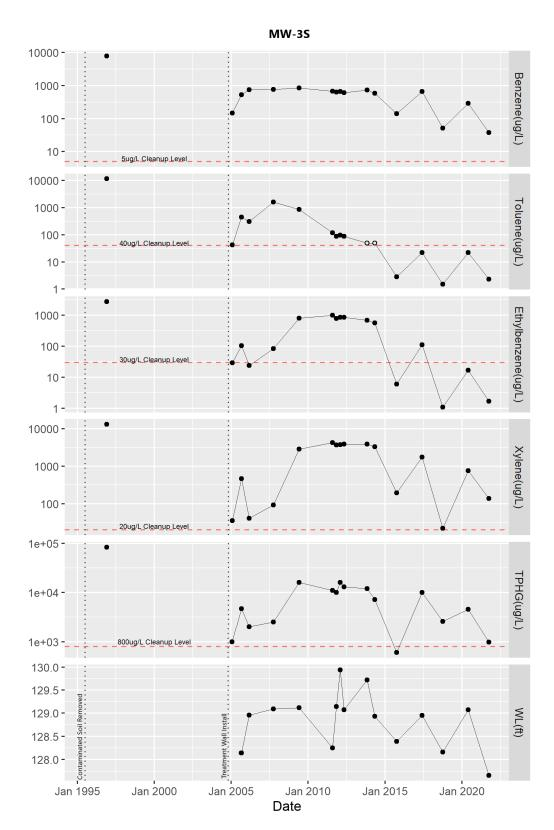
Figure A3. Contaminant concentrations (µg/L, log scale) and groundwater elevations (ft) for well MW-3S, November 1993 to October 2021. Open circles indicate analyte was not detected and are plotted at one-half the reporting limit.
