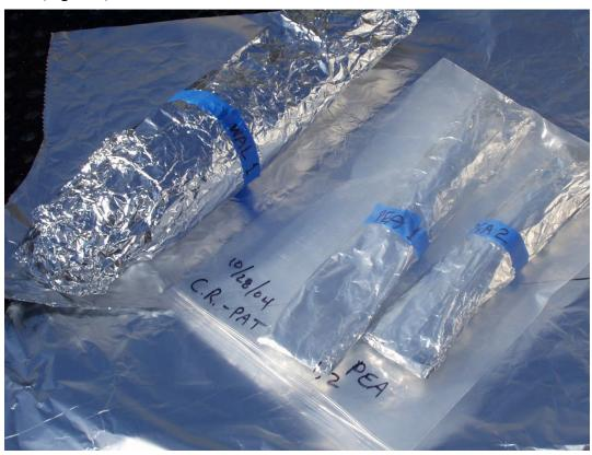
Figure 9 Fish wrapped in two layers of foil (dull side to fish), taped with label and placed with same species into labeled watertight polyethylene bags.
