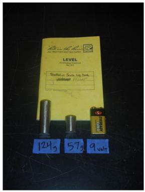
Figure 4 Scale Log Book, Standard Weights, 9-volt battery (Items stored in scale case).
