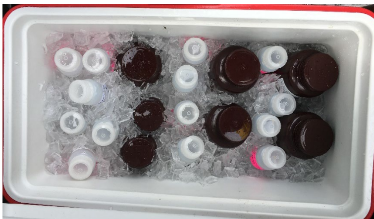
Figure 3. Particulate sample bottles (organic carbon and nitrogen, total organic carbon and total nitrogen) in coolers for transit.
