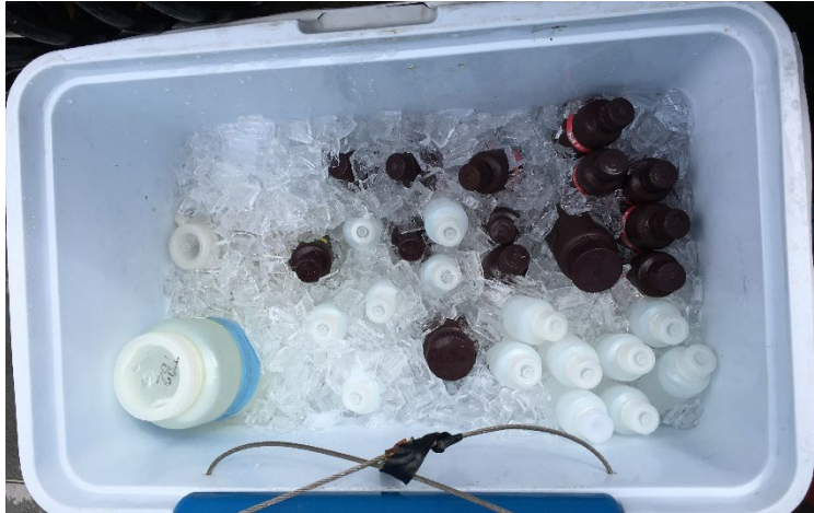
Figure 4. Chlorophyll a and nutrient bottles in coolers for transit.
