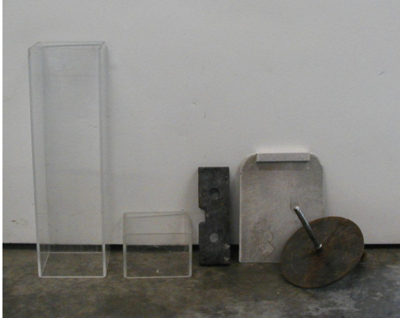
Figure 2. Pictured left to right acrylic liner (50 cm), acrylic liner section, lead weight, slicing plate, and hand crank.
