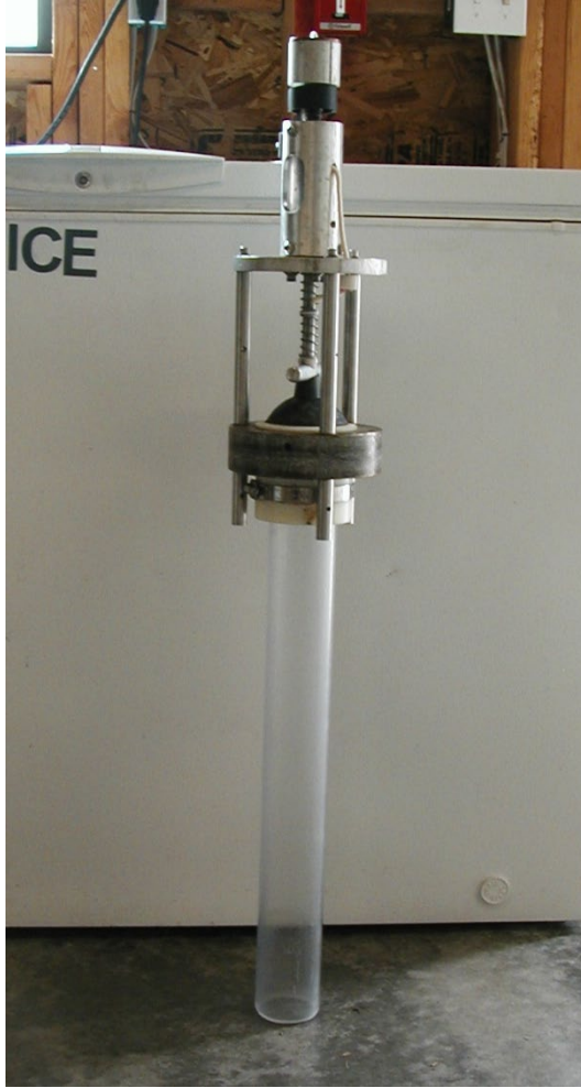
Figure 4. Modified KB corer with suction cup engaged.
