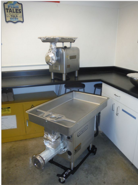
Figure 4. Hobart grinding units (small unit #4812, large unit #4732A)..
