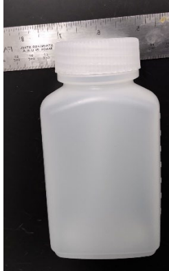
Figure 2. PFAS sample container; CapSure oblong HDPE WM.
