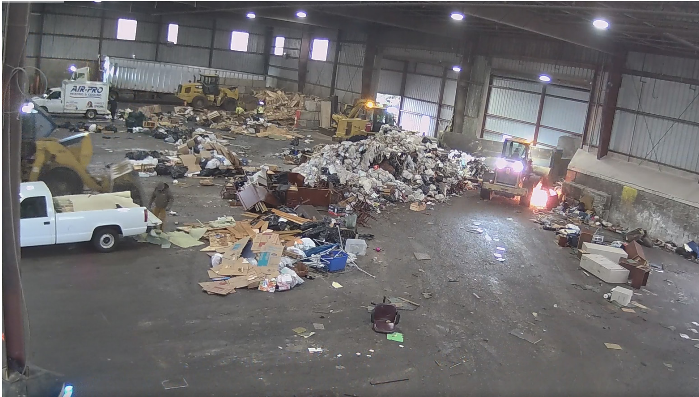
An example of a fire in a warehouse caused by a lithium-ion battery.
