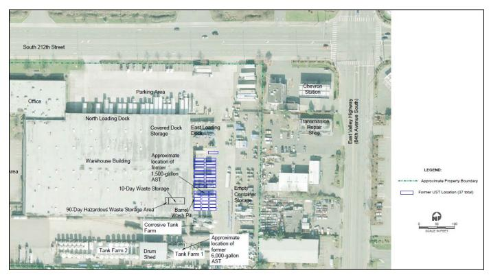
Figure 3: Tank farm locations at Univar, including 2 aboveground storage tanks and 37 underground storage tanks (outlined in purple). Source: Univar's RCRA Corrective Action Permit Renewal Application, Part A and B.
