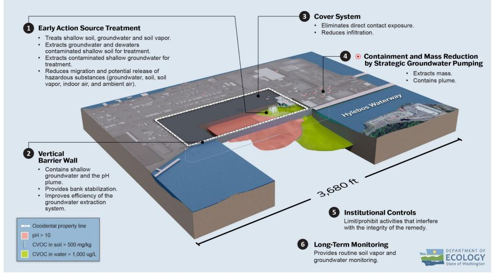
Figure 2. Key elements of the Occidental site cleanup plan. (CVOC = chlorinated volatile organic compounds.)
